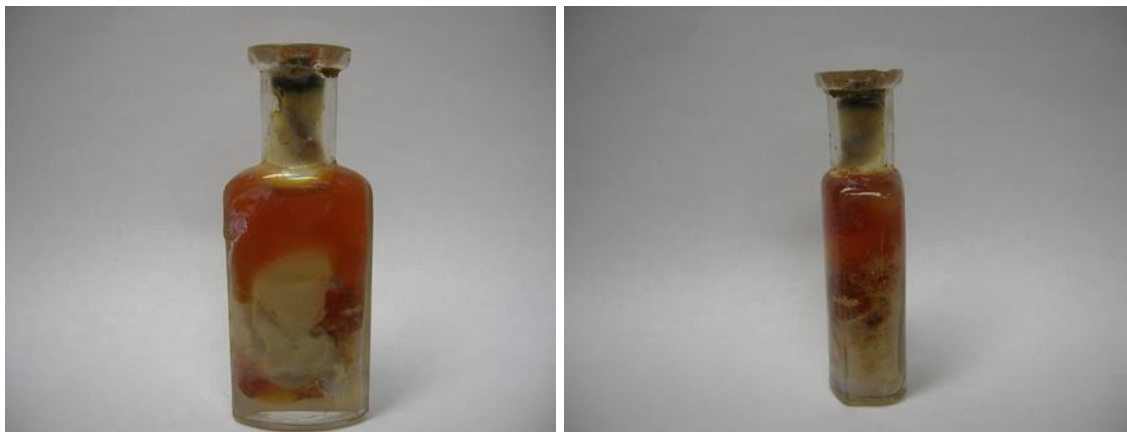
Fig.5 – Unopened sample bottle: Separation of the contents had occurred while in the well. The cork had degraded but appeared to have retained the majority of the original contents without too much contamination. The oil helped to repel water and maintain sample integrity. The two sample components were analyzed separately but mixed easily into a light yellow, oily paste.
