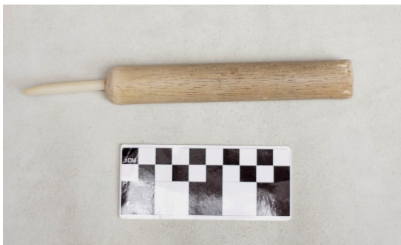
Figure 20b. Bone pressure flaker in wood handle use in crystal tool edge refinement.
