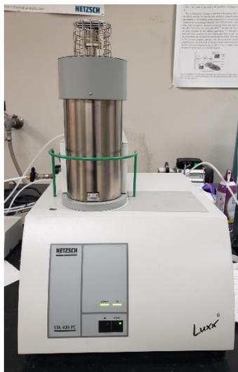
Figure 4.1 Netzsch TGA-DSC instrument
