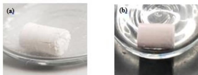
Figure 3.18 Pellet after the first decomposition of  $\text{Ca(OH)}_2$ : (a) pure  $\text{Ca(OH)}_2$ , (b) composite pellet
