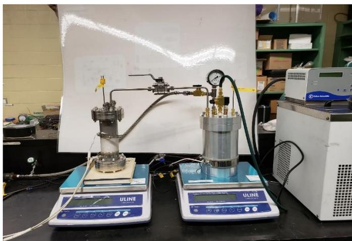
Figure 4.3 Lab scale experimental setup (left side: chemical reactor; right side: condenser/evaporator)
