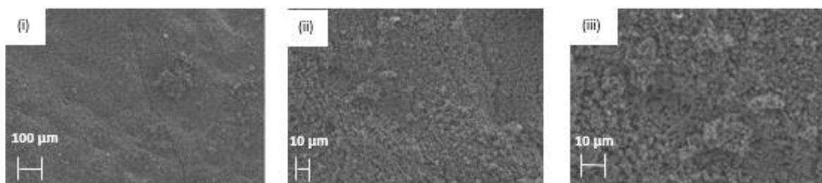
Figure 4.13 SEM images after 1<sup>st</sup> dehydration reaction at magnification (i) 100 X (ii) 500 X (iii) 1000 X
