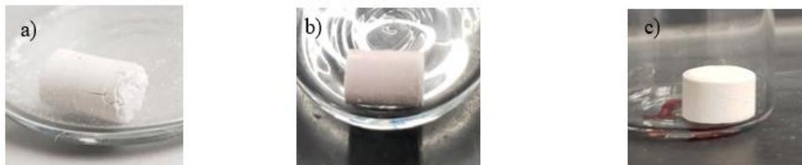
Figure 4.30 Pellet after the first decomposition of  $\text{Ca(OH)}_2$ : (a) pure  $\text{Ca(OH)}_2$ , (b) composite pellet and c) after 20 cycles
