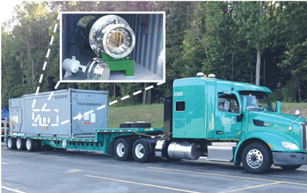
Figure 5.5: NAC LWT fully assembled
