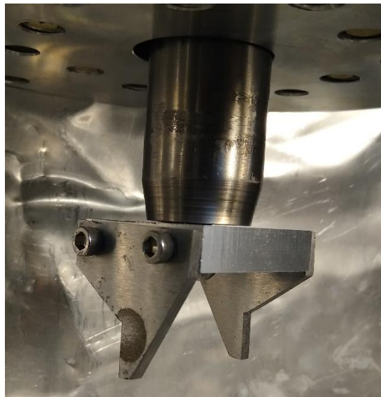
Figure 3.9. Rotary scraper dynamometer head.
