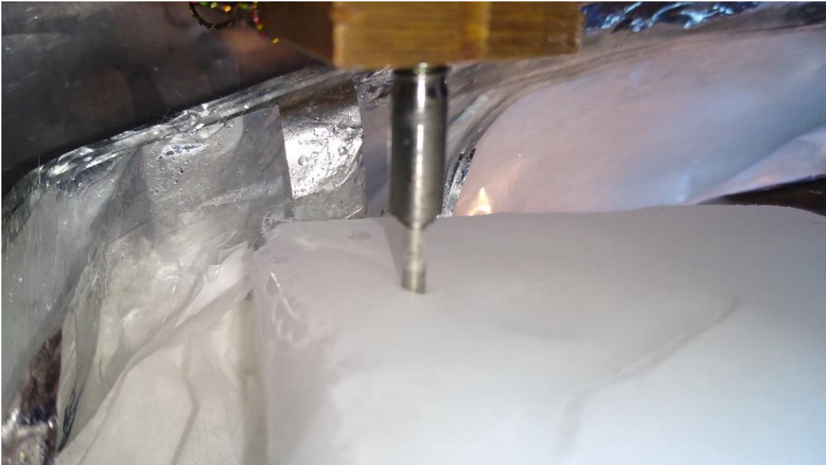
Figure 4.1. Indenter collecting data on dry ice.
