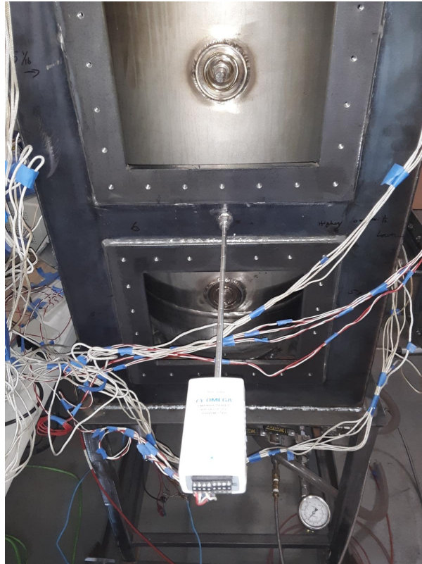
Figure 5.5: The hot wire anemometer housing on the left side of the RPV containment structure.
