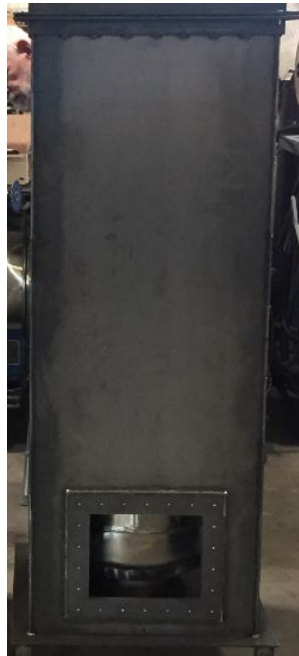
(b) The PGV containment structure with the vessel inside.
