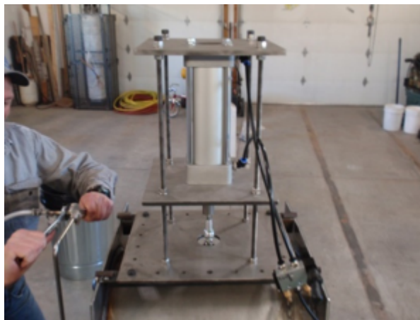
Figure 3.19: Testing the pneumatic ram.
