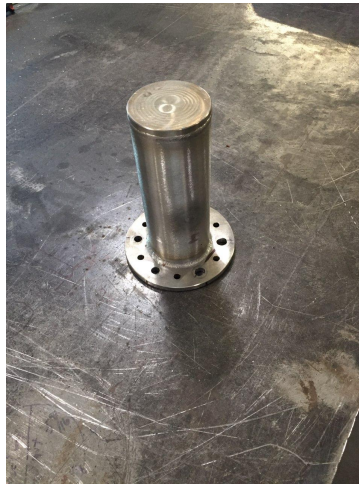
(b) The outside of the oxygen sensor shaft housing.
