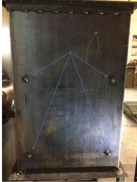
Figure 5.2: Thermocouple locations, as indicated by blue arrows, on the back side of the RPV containment structure.
