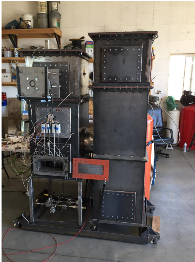
Figure 3.1: The assembled \frac{1}{20} th scaled model of a VHTR.
