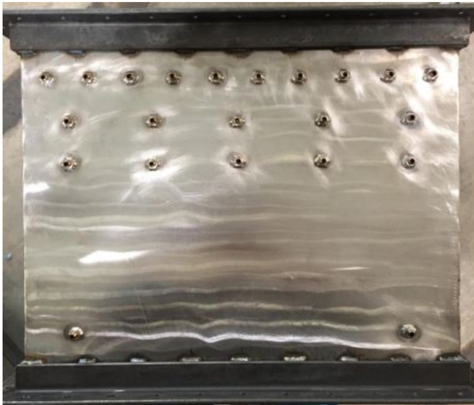
Figure 3.21: Thermocouple and heating cartridge wire locations on the back side of the top of the RPV containment structure.
