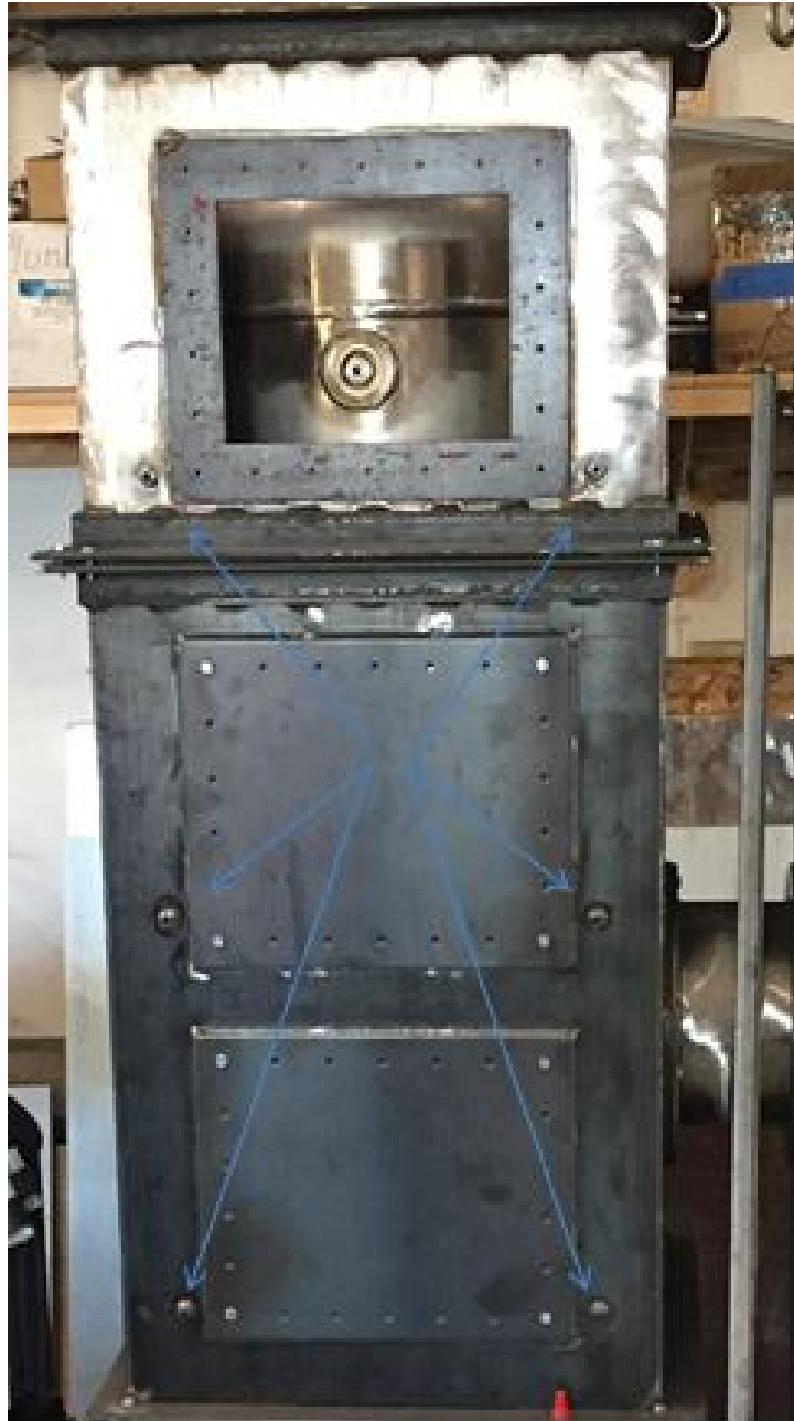
Figure 5.1: Thermocouple locations, as indicated by blue arrows, in the RPV containment structure.
