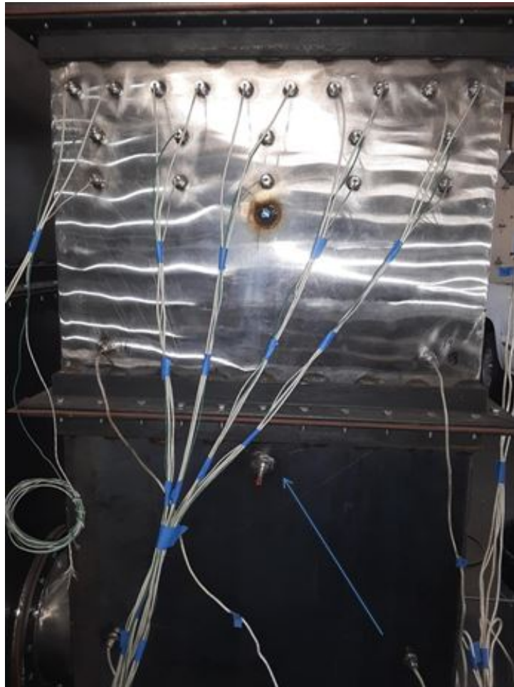
Figure 5.6: The hot wire anemometer housing, as indicated by a blue arrow, on the back side of the RPV containment structure.
