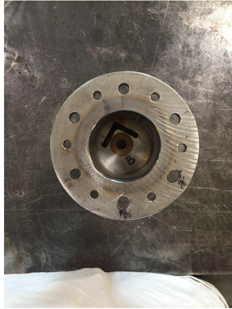
(a) The grooves for the all thread and angle iron inside of the oxygen sensor shaft housing.
