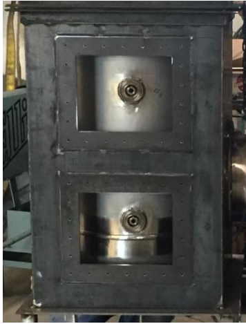
(b) The pressure vessel containment structure with the pressure vessel inside.
