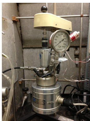
Figure 2.1 Parr reactor setup and the applied parameters during hydrotreatment of phenol
