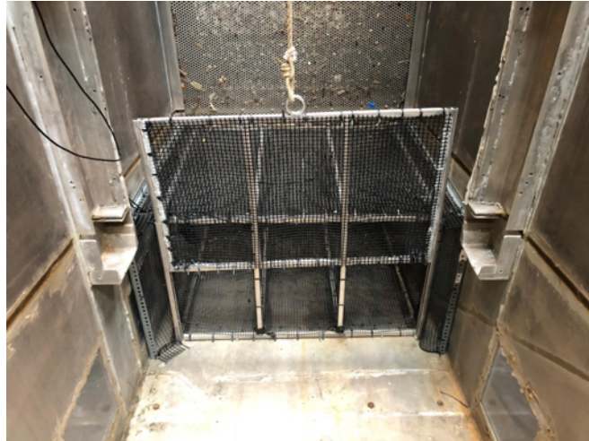
Figure 1.1 Mesh exercise chamber located in the downstream portion of the experimental flume
