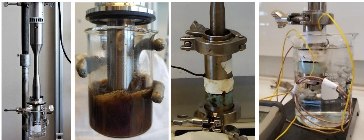
Figure 3.4. Ultrasonic-assisted catalytic transfer hydrogenation.
