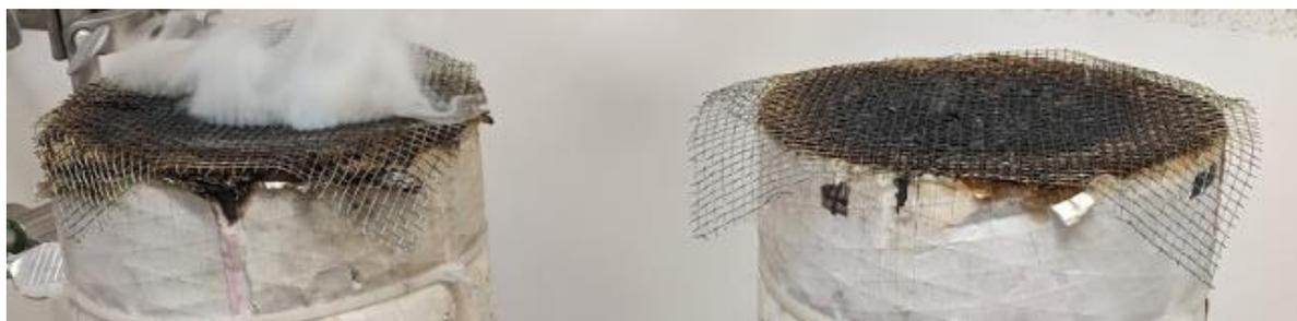
Figure 2.10: Spark arrestors installed on two reactors. The left reactor is under spontaneous combustion at 5 L/min airflow, but no flame was present.
