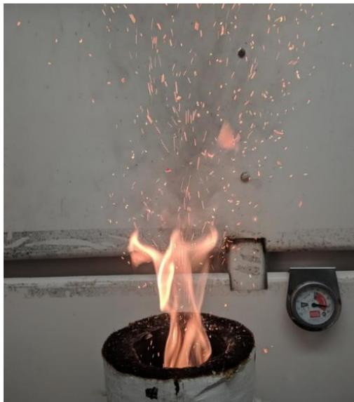
Figure 2.9: Potentially dangerous sparks leaving an ignited reactor under airflows greater than 5 L/min.
