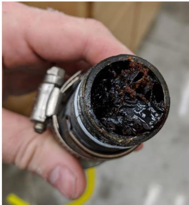
Figure 2.17: Excessive oils dripped down into the heating core, causing a polymer to form which greatly restricted airflow and reactor performance.
