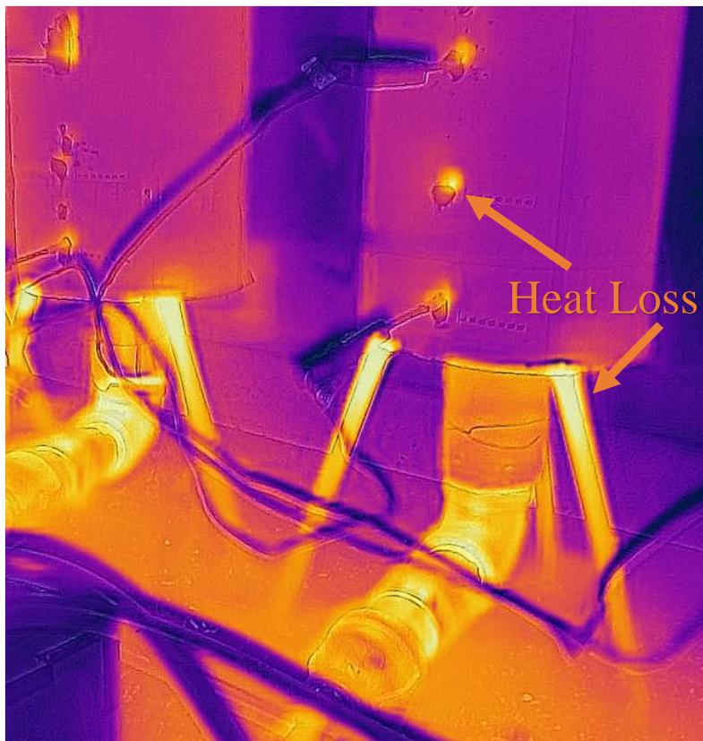
Figure 3.3: Thermal image of reactors during operation. Heat loss is seen in the legs of the reactors and through the holes for thermocouples. Reactor 4 has four holes for extra temperature measurement locations
