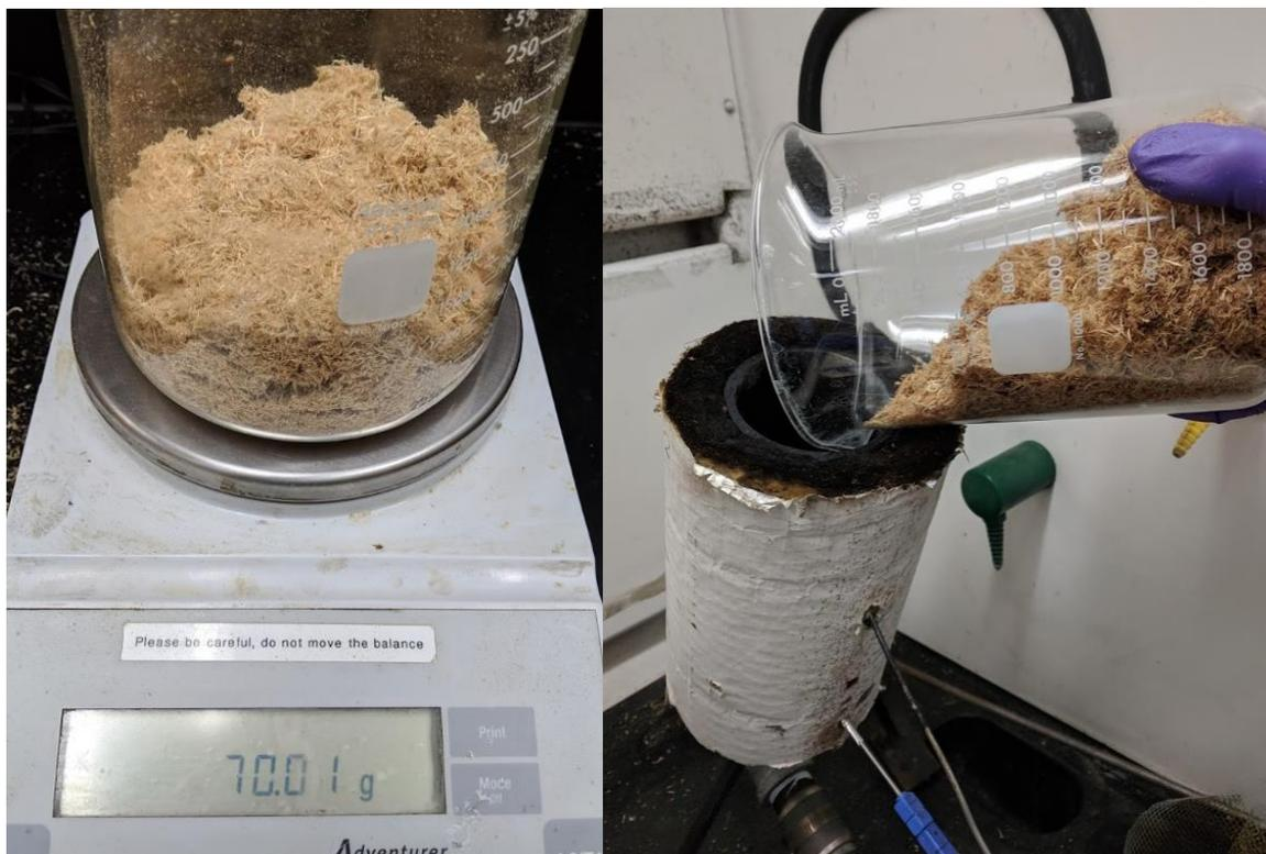
Figure 2.14: Sawdust weighed on a digital scale for each reaction (left). After mixing test chemicals in the sawdust, it is added to the reactor by pouring in the top.
