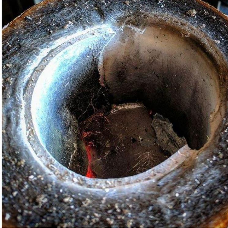
Figure 2.3: Melted aluminum reactor on a glowing bed of smoldering sawdust.
