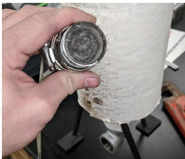
Figure 2.6: Steel wool stuffed steel pipe wrapped in a 160W mica band heater.
