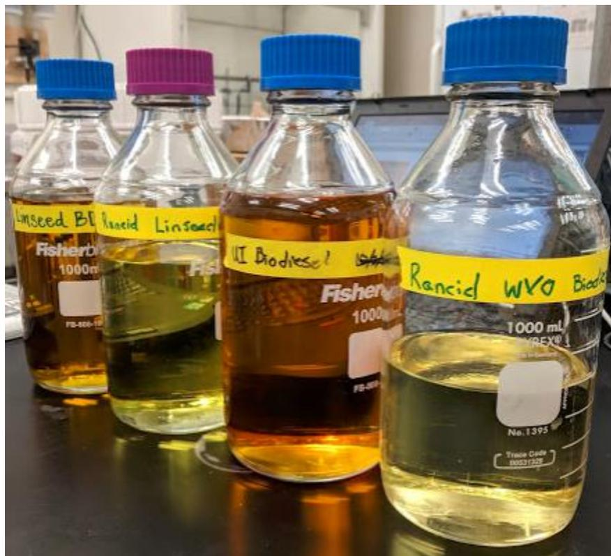
Figure 2.1: Rancid and Fresh versions of prepared biodiesel for testing. From left to right: Linseed Biodiesel, Rancid Linseed Biodiesel, Biodiesel from WVO and Rancid Biodiesel from WVO. The rancid biodiesel had a lighter color than the fresh biodiesel.
