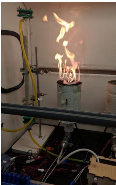
Figure 2.8: Planned worst-case scenario testing in a laboratory hood. Max pressure and max airflow were forced through heavily oil-saturated sawdust and ignited. No damages were observed to hood or equipment.
