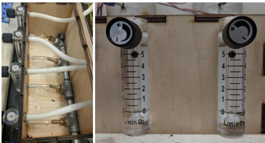
Figure 2.12: Compressed air manifold (left) and airflow metering valves (right).
