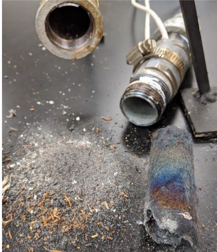
Figure 2.15: Excessive ash buildup in the bottom of the reactor reduced airflow and reactor performance. Thermal coloring of the steel wool shows cooler temperatures farthest from the mica heating band indicating effective heat transfer to air.
