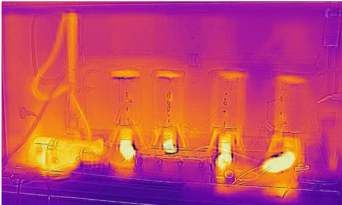
Figure 3.5: Thermal image of the experimental setup during operation. Reactors are numbered from left to right, 1 to 4 respectively. Reactor 1 and 2 were slightly closer together in position and in close proximity to the compressor.
