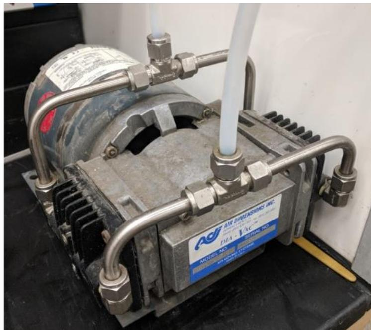
Figure 2.11: Dia-Vac continuous use air compressor to ensure consistent air supply.
