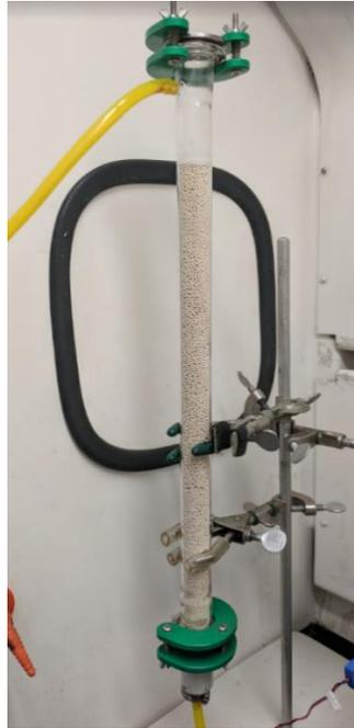
Figure 2.13: A4 molecular sieve air dryer to remove atmospheric water.
