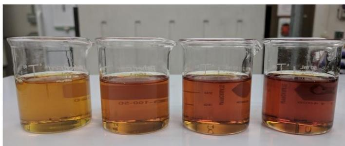
Figure 2.20: Increasing amount of Ethanox 4760R, in boiled linseed oil with the leftmost not containing any antioxidant followed by 0.06%, 0.12% and 0.2% of antioxidants by mass.
