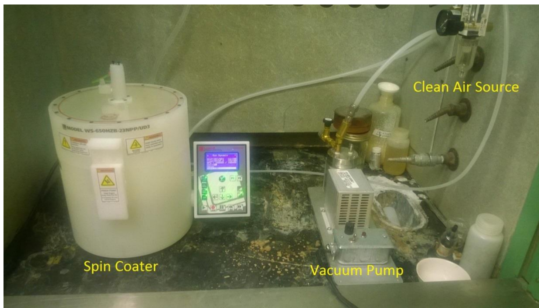
Figure 2.1. Laurell Technologies spin coater setup.
