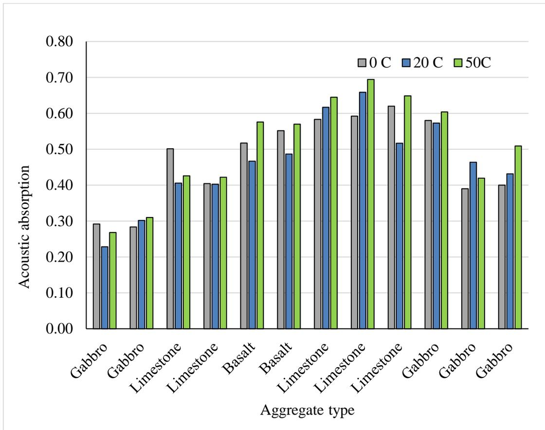
**Figure 4.34** Absorption coefficient of asphalt samples at different temperature
