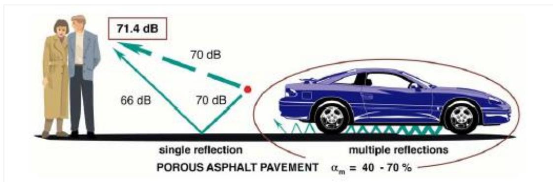
**Figure 2.8** Sound absorption into a porous asphalt pavement (Sandberg and Ejsmont 2002)
