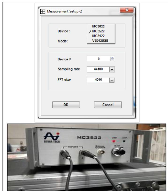
**Figure 3.12** Sound card setting with MC 3522 channel
