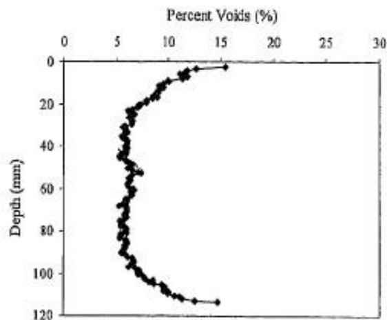
**Figure 4.36** Air void distribution in superpave gyratory compactor (SGC) and linear kneading compactor (LKC) specimens (after Masad et al. 1999)
