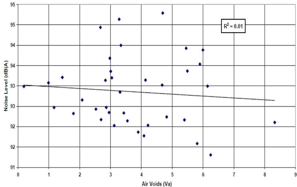
**Figure 2.10** Effect of air voids on tire/pavement noise for dense graded HMA Mix (Hanson et al. 2004).
