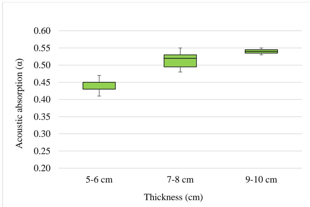
**Figure 4.12** Box plot of acoustic absorption of pavement for different thickness (Basalt)
