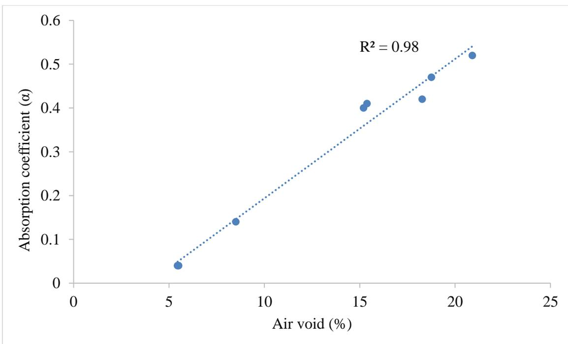
**Figure 4.8** Correlation between acoustic absorption of pavement and air void (Limestone)
