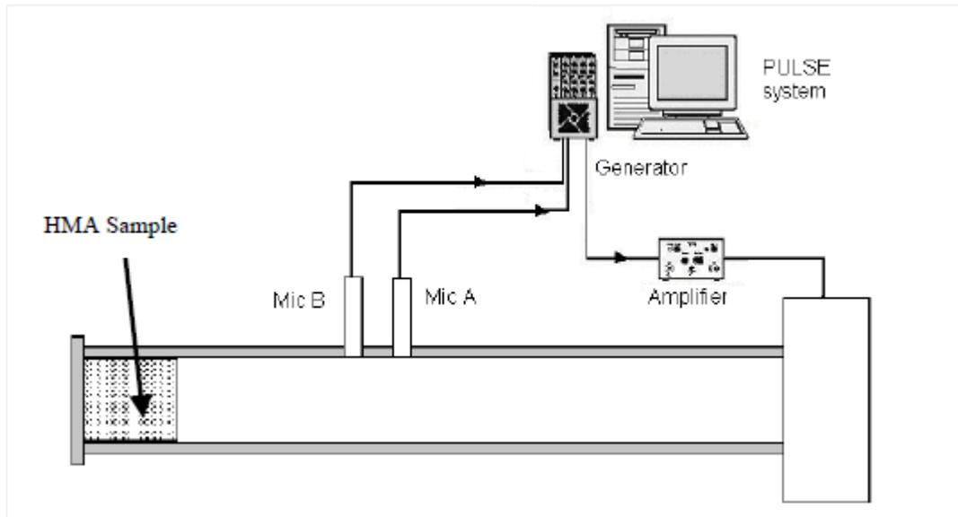
**Figure 2.11** Experimental setup of sound absorption of HMA samples (Hanson et al. 2004)
