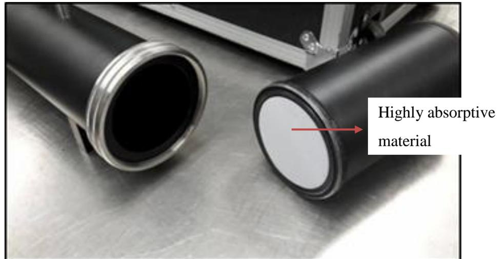
**Figure 3.15** Highly absorptive material inside the sample holder.
