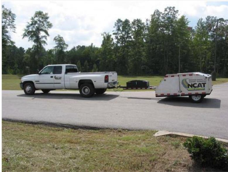
**Figure 2.4** NCAT close proximity trailer (Hanson et al. 2004)
