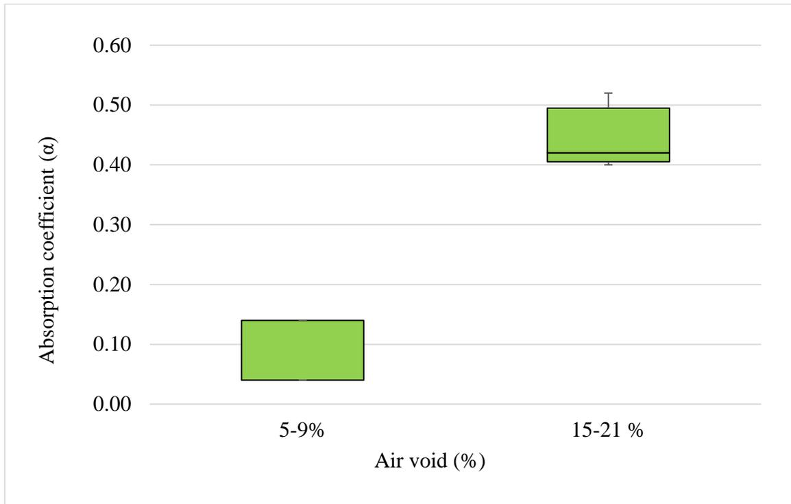
**Figure 4.7** Box plot of acoustic absorption of pavement for different air void (Limestone).
