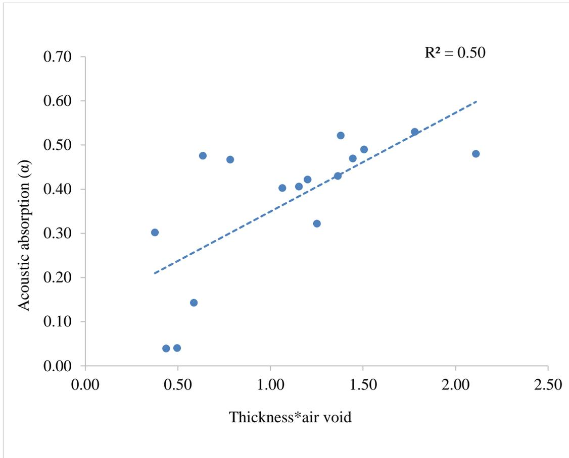
**Figure 4.16** Correlation between acoustic absorption of pavement and thickness x air void (Limestone)
