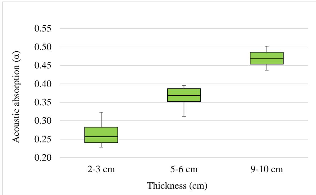
**Figure 4.10** Box plot of acoustic absorption of pavement for different thickness (Gabbro)
