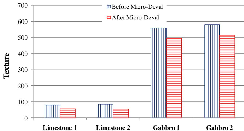
**Figure 3.6** Average texture index before and after the micro-deval test (Masad et al. 2011)
