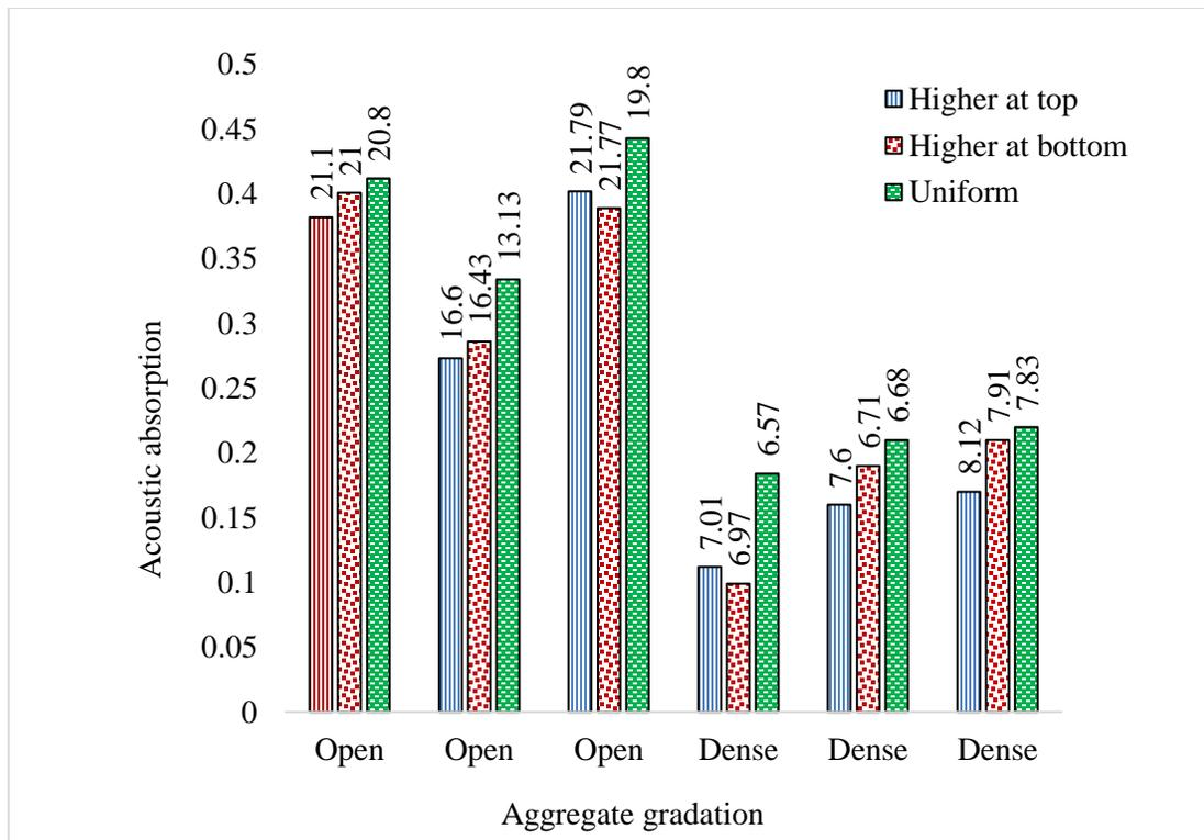
**Figure 4.37** Absorption coefficient of asphalt samples for different air void structure
