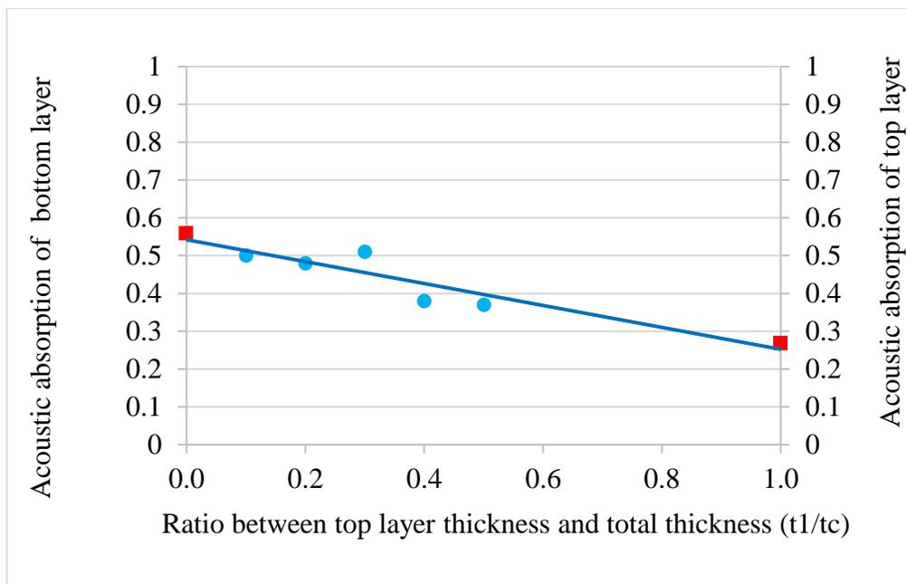
**Figure 4.30** Change in absorption coefficient with the change in thickness ratio of the top and bottom layer of a double layer
