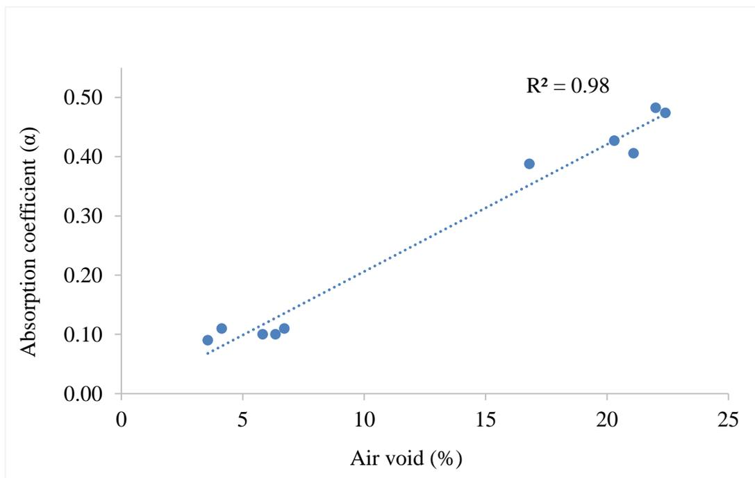
**Figure 4.4** Correlation between absorption coefficient of pavement and air void (Gabbro)
