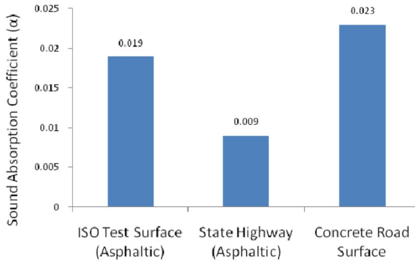
**Figure 2.7** Comparison of sound absorption coefficients of three different road surfaces
