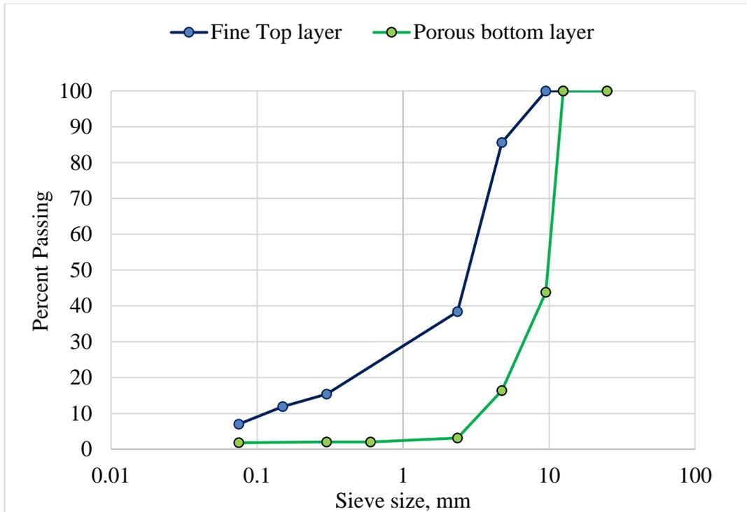
**Figure 4.29** Gradation of top and bottom layer for the double layer pavement
