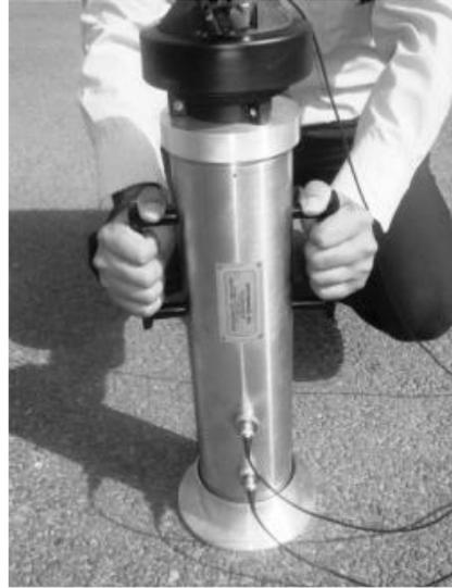
**Figure 2.6** In-situ measurement of road sound absorption coefficient by impedance tube
