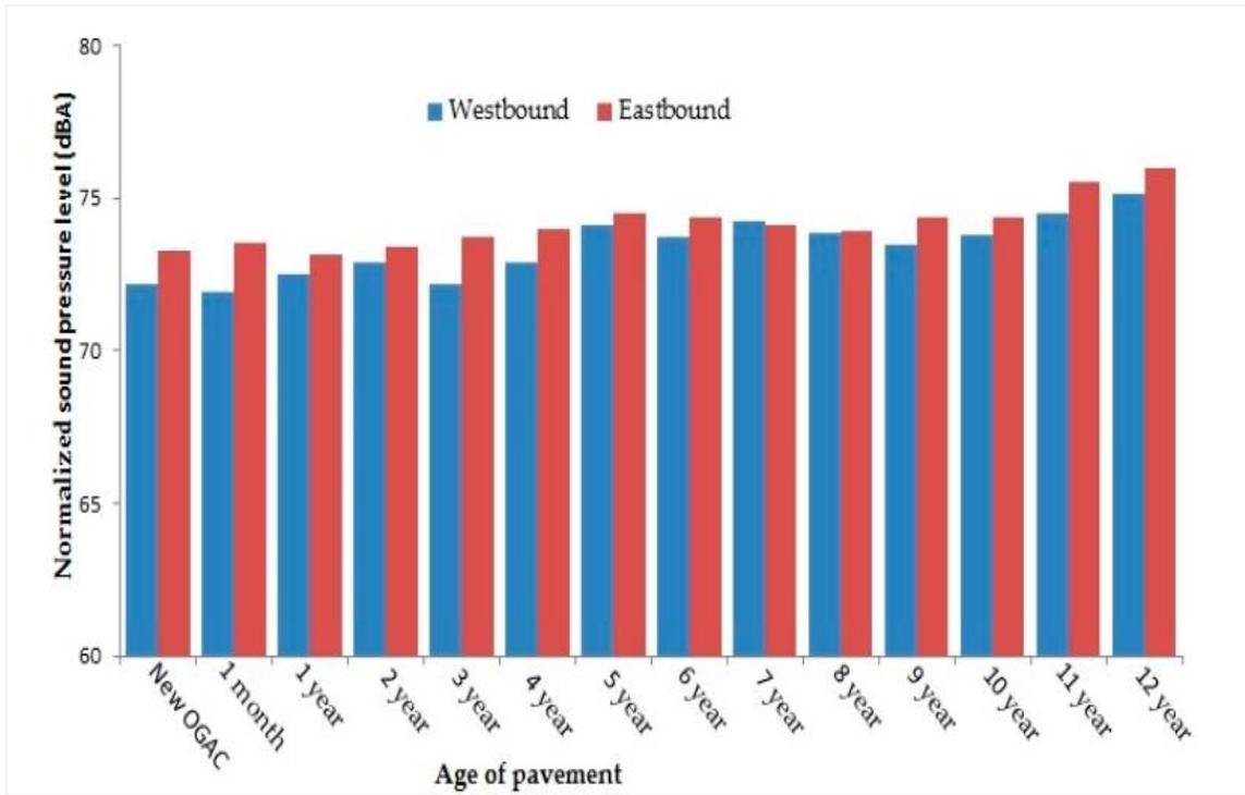
**Figure 2.16** Noise level measurement using CTIM method (Illingworth & Rodkin, Inc 2011).
