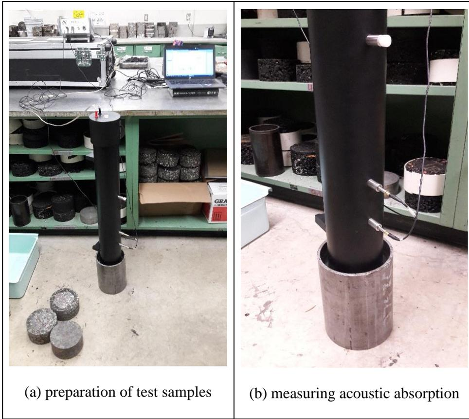
**Figure 3.17** Acoustic absorption measurement
