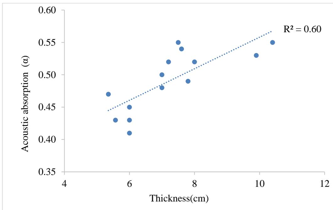
**Figure 4.13** Correlation between acoustic absorption of pavement and thickness (Basalt)
