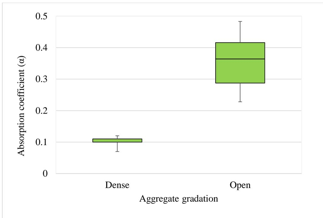
**Figure 4.2** Boxplot of acoustic absorption of pavement for dense-graded and open-graded mixture
