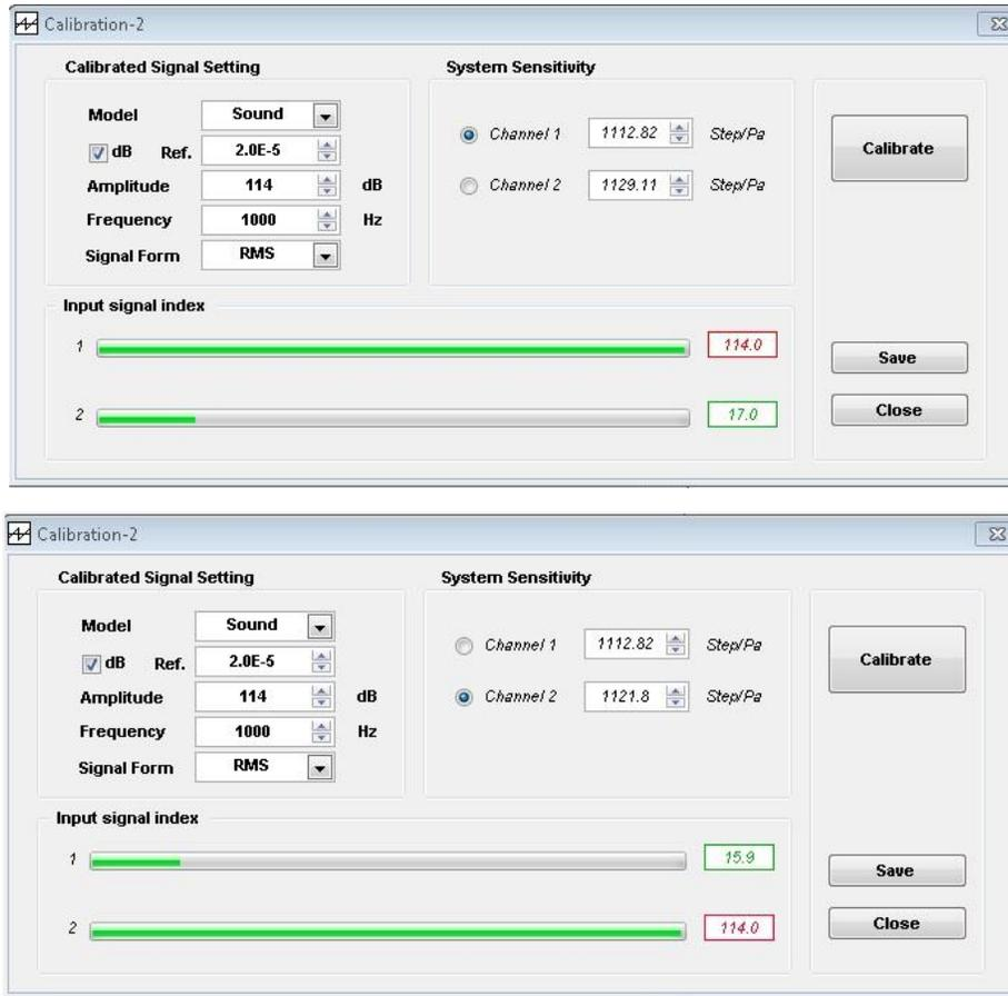
**Figure 3.14** Microphone calibration window for channel 1 and channel 2.
