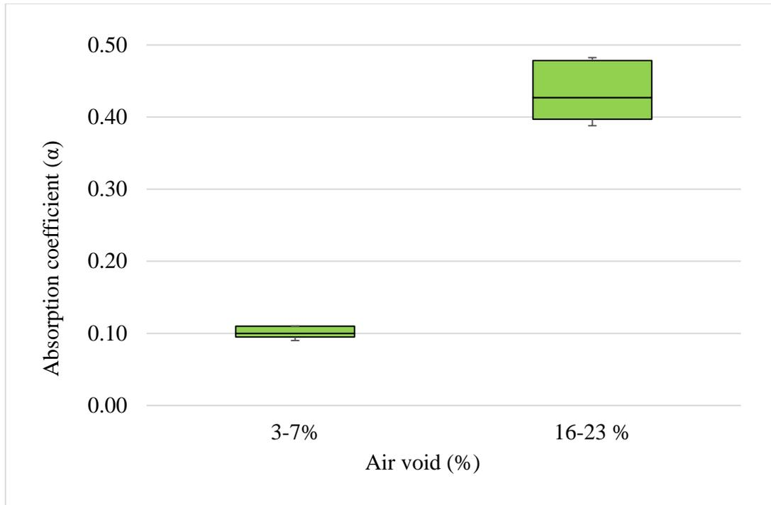
**Figure 4.3** Box plot of absorption coefficient of pavement for different air void (Gabbro).
