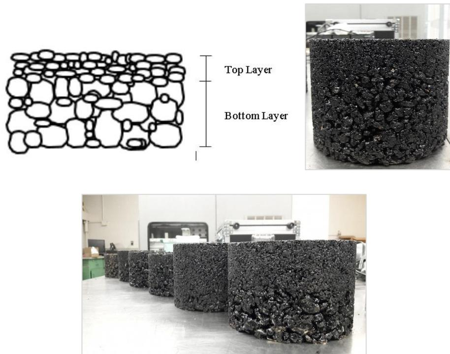
**Figure 4.28** Double layer test samples
