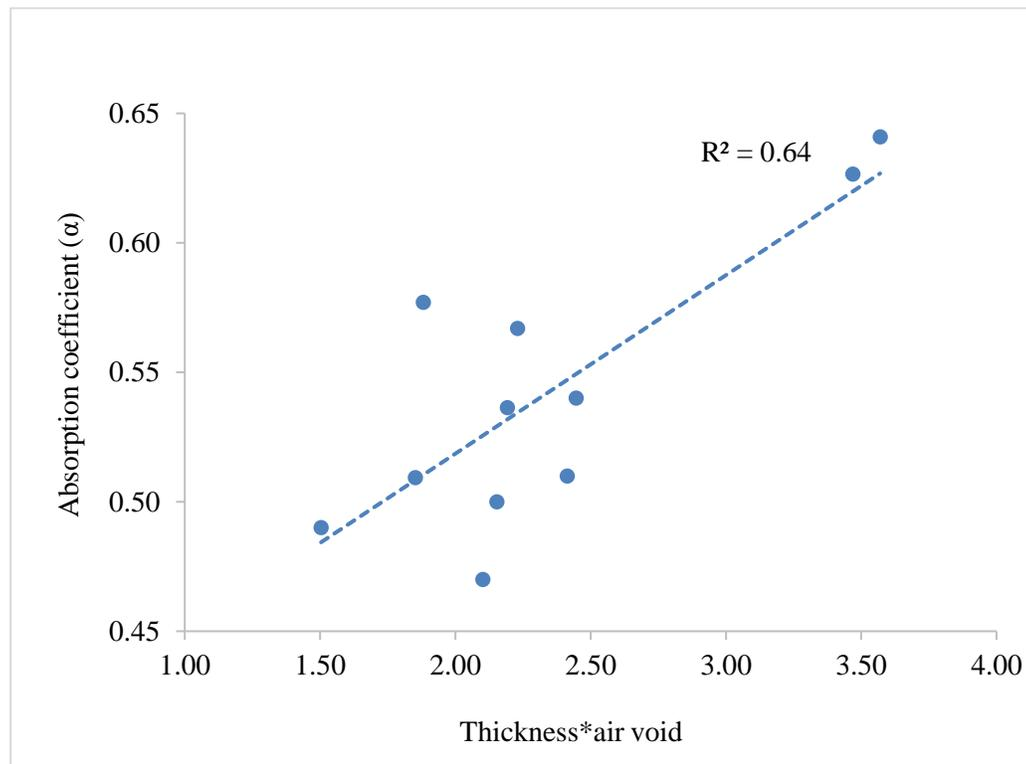
**Figure 4.17** Correlation between acoustic absorption of pavement and thickness x air void (Lightweight)
