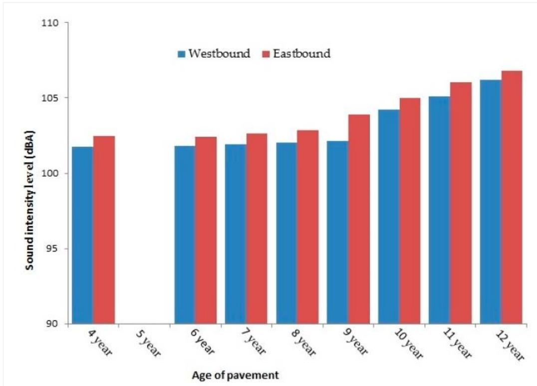
**Figure 2.17** Noise level measurements using OBSI method (Illingworth & Rodkin, Inc 2011)
