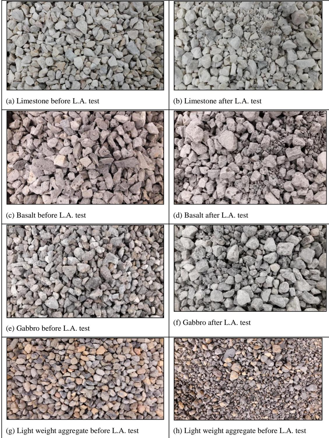
**Figure 3.2** Aggregate before and after abrasion test
