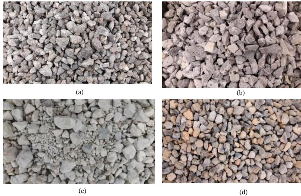
**Figure 4.19** Different types of aggregates, (a) gabbro, (b) basalt, (c) limestone, and (d) lightweight
