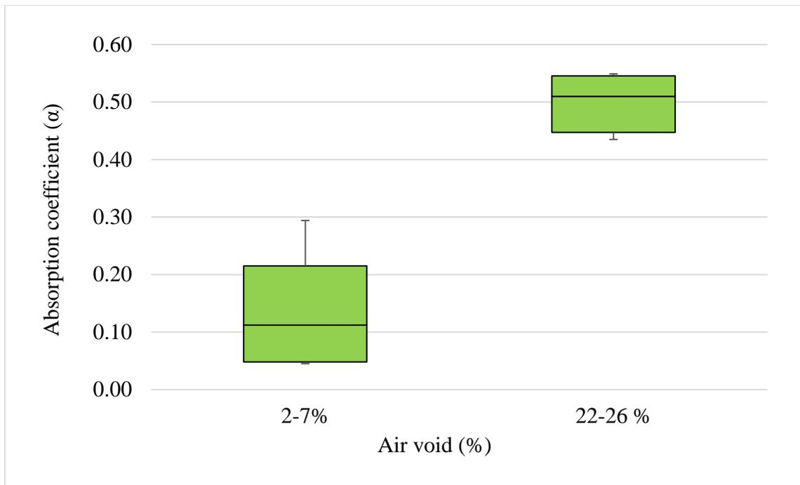
**Figure 4.5** Box plot of absorption coefficient of pavement for different air void (Basalt).
