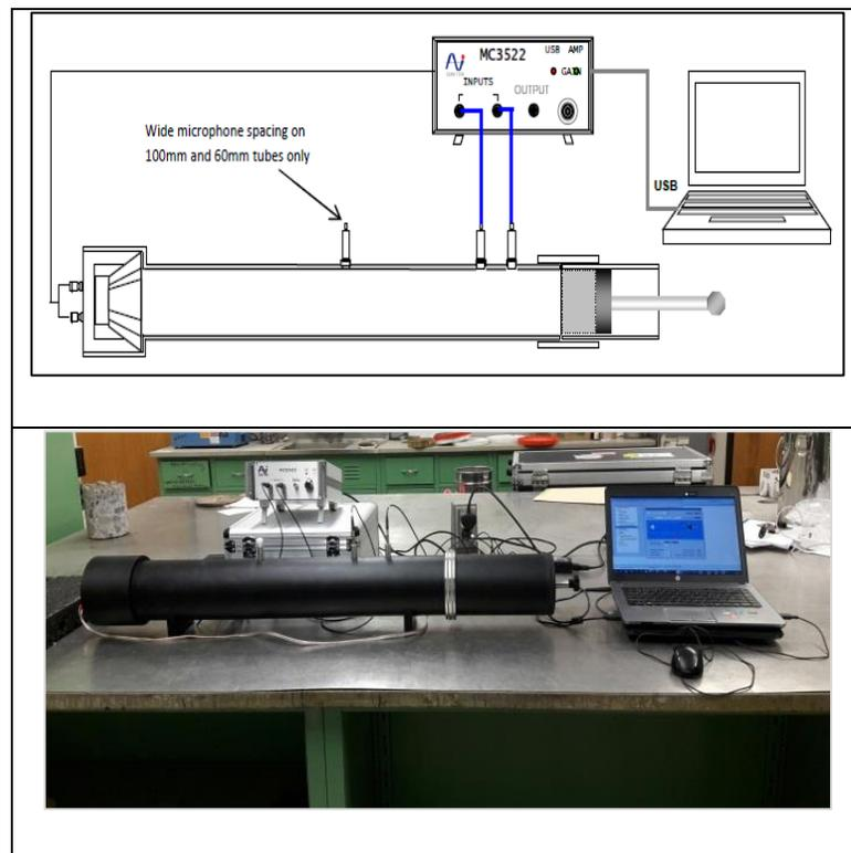
**Figure 3.11** Impedance tube set-up
