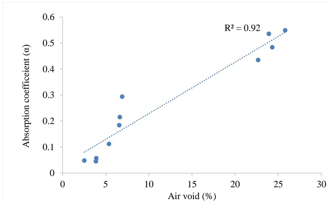
**Figure 4.6** Correlation between acoustic absorption of pavement and air void (Basalt).
