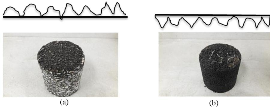
**Figure 4.38** Surface texture, (a) Positive, and (b) Negative
