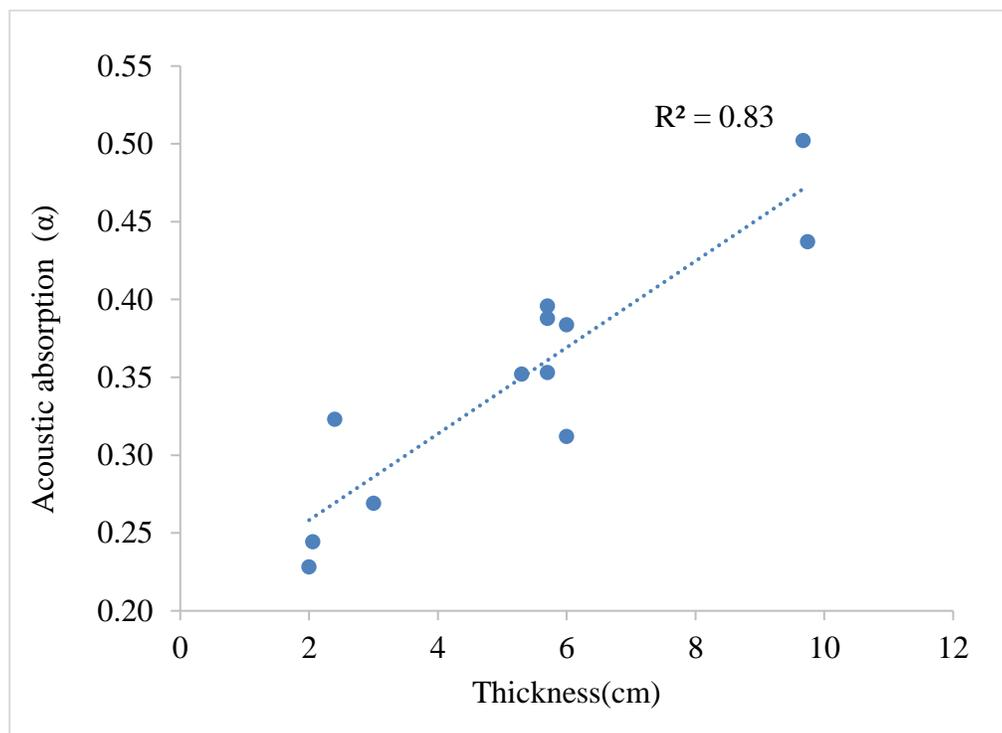
**Figure 4.11** Correlation between acoustic absorption of pavement and thickness (Gabbro)
