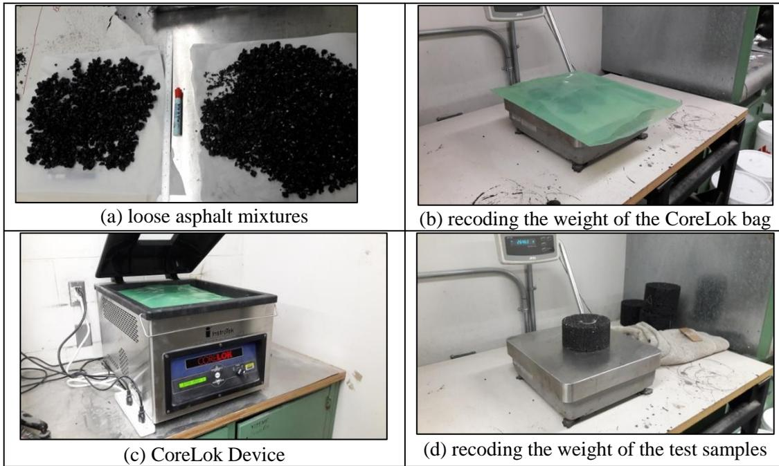
**Figure 3.10** Air void measurement in the laboratory
