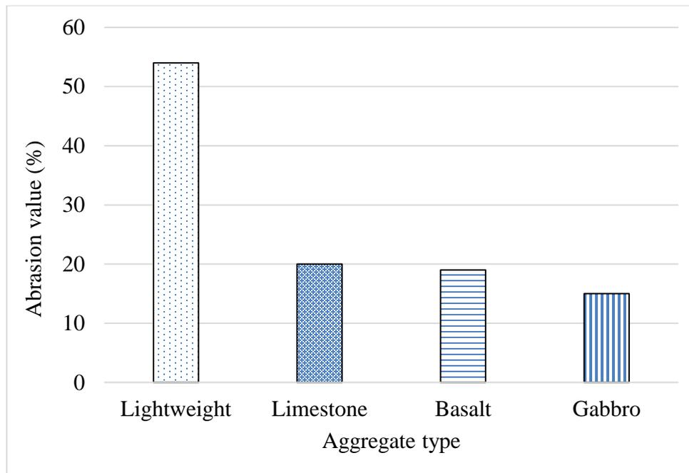
**Figure 3.3** Abrasion value for different types of aggregate.
