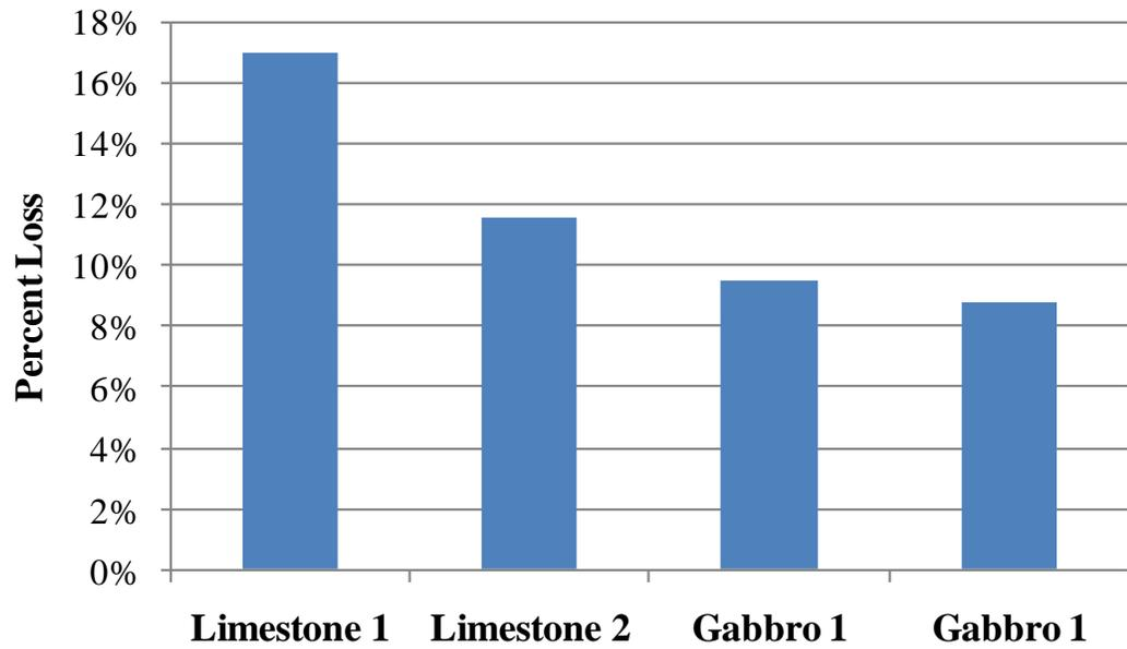
**Figure 3.5** Micro-Deval abrasion loss (Masad et al. 2011)
