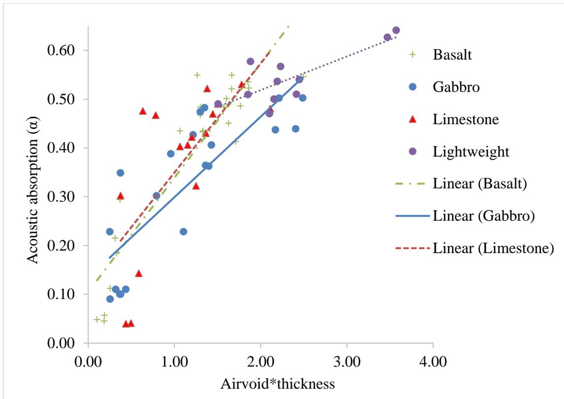
**Figure 4.18** Correlation between acoustic absorption of pavement and thickness x air void
