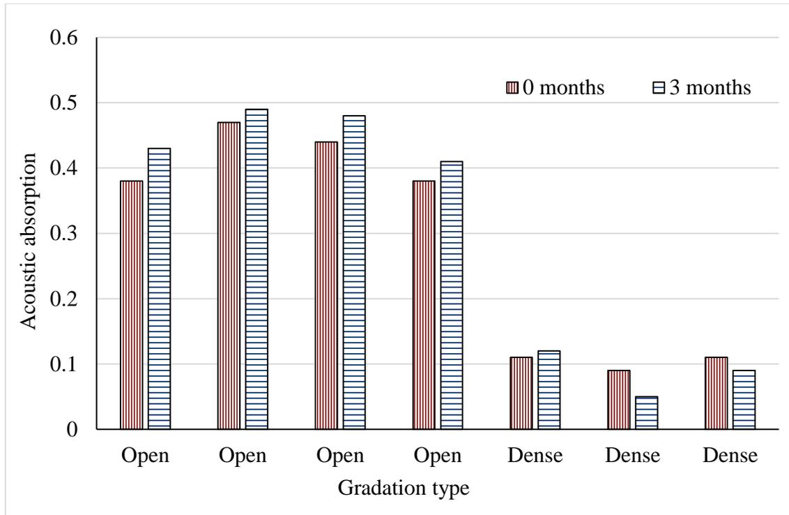
**Figure 4.32** Effect of aging on absorption coefficient
