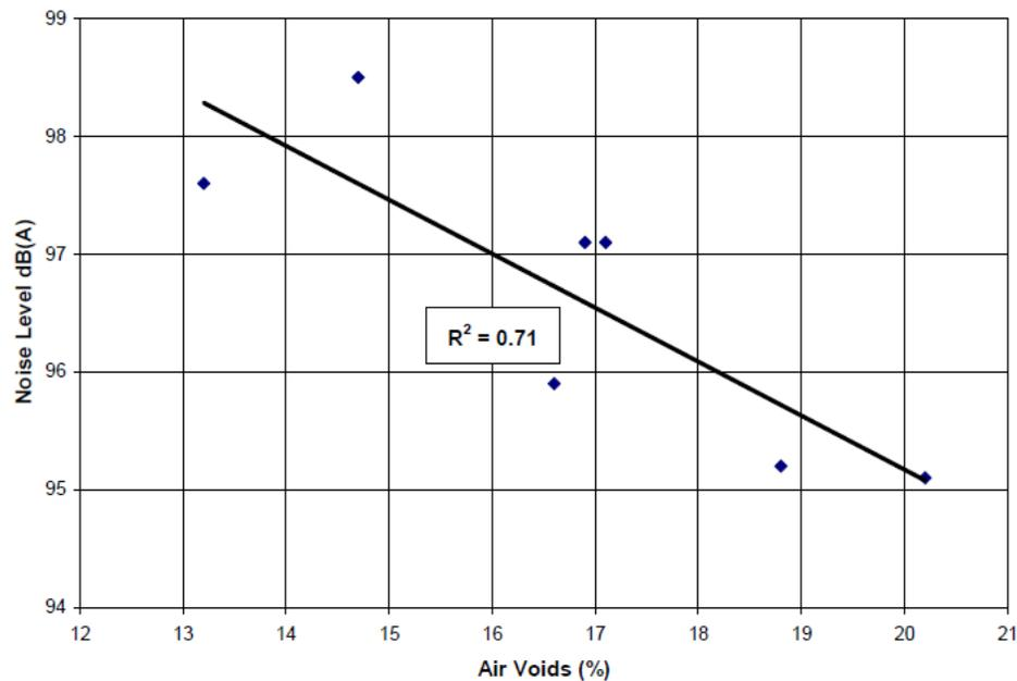
**Figure 2.9** Effect of air void on noise level of OGFC (Hanson et al. 2004)
