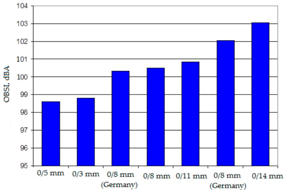
**Figure 2.20** Noise performance of stone mosaic asphalt (SMA) pavements of varying aggregate size for four European countries (Donavan 2006)
