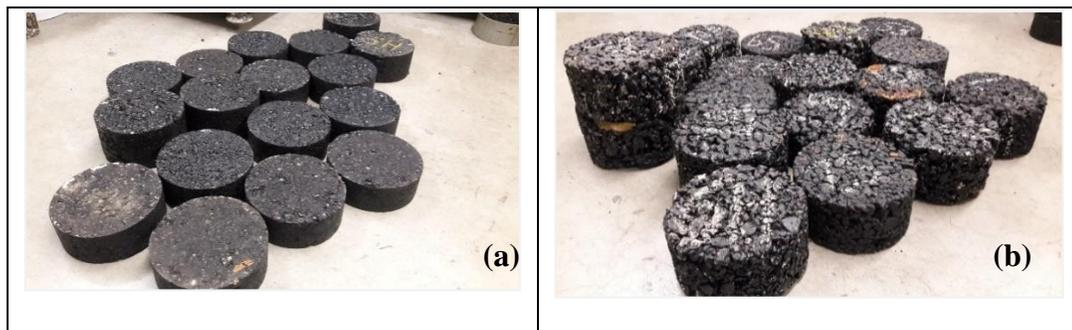
**Figure 4.1** Asphalt samples of different aggregate gradation (a) well-graded and (b) open-graded
