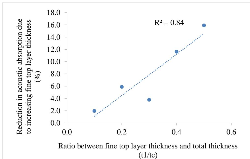
**Figure 4.31** Reduction in acoustic absorption due to increase of top layer thickness of a double layer
