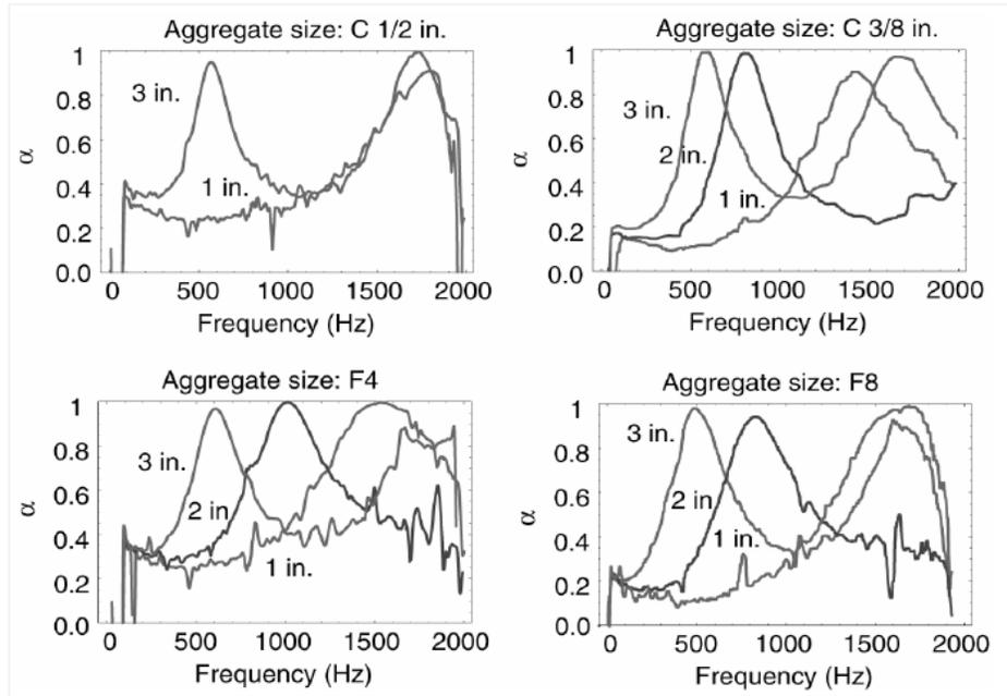
**Figure 2.14** Effect of thickness on acoustic absorption (DeMoss et al. 1999)
