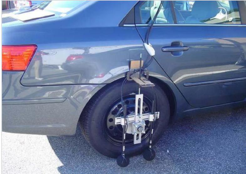
**Figure 2.5** OBSI testing setup
