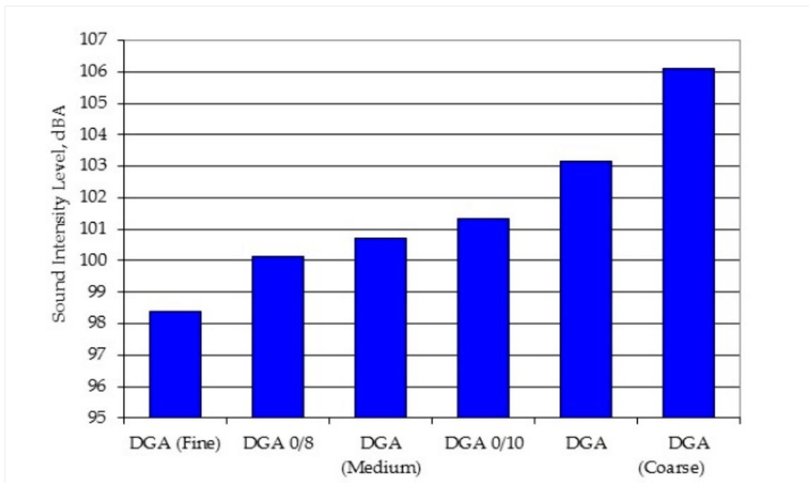
**Figure 2.19** Noise performance of dense graded asphalt (DGA) pavements of varying aggregate size for four European countries (Donavan 2006)
