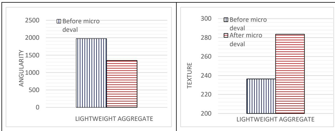
**Figure 3.8** Average angularity index for lightweight aggregate before and after the micro-deval test
