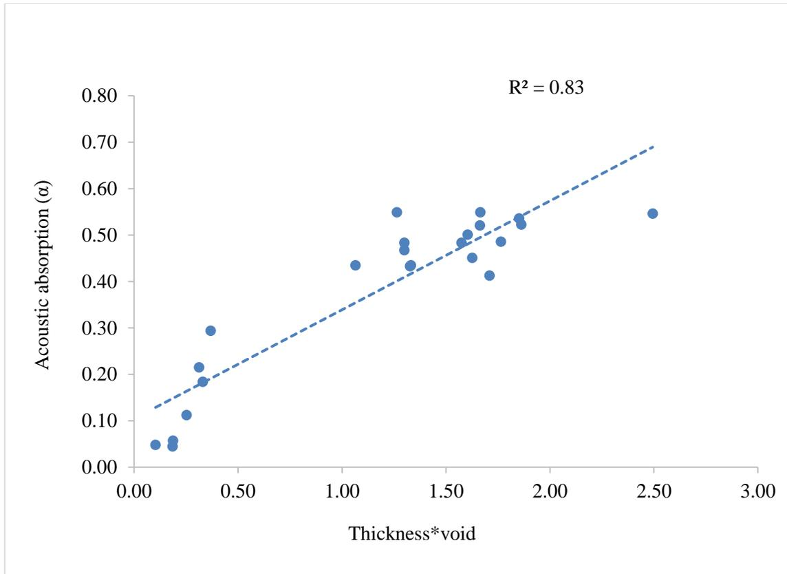
**Figure 4.15** Correlation between acoustic absorption of pavement and thickness x air void (Basalt)
