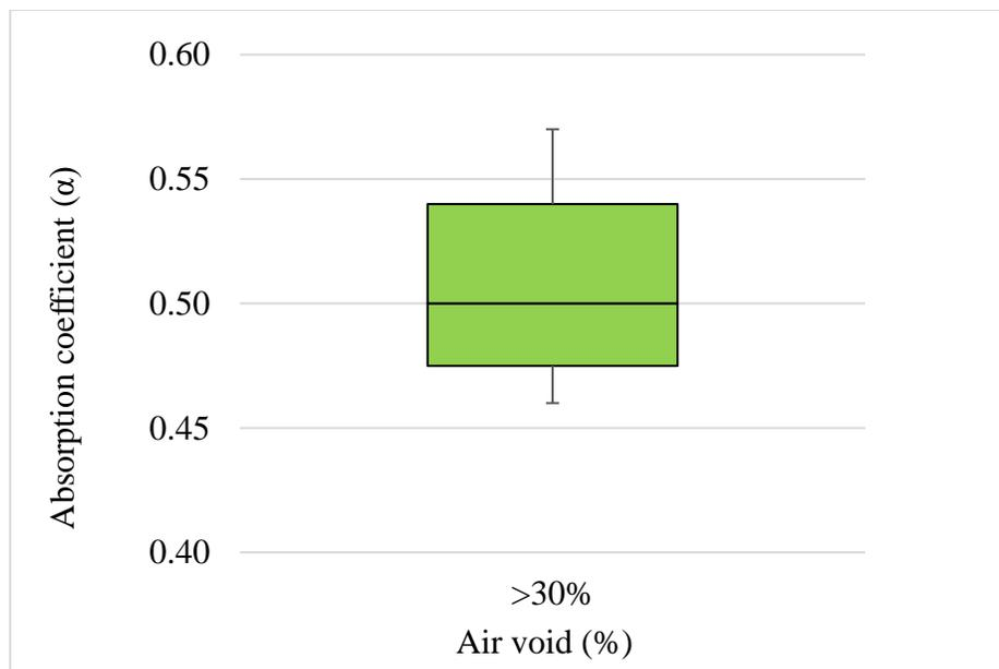
**Figure 4.9** Box plot of acoustic absorption of pavement for higher air void (Lightweight)
