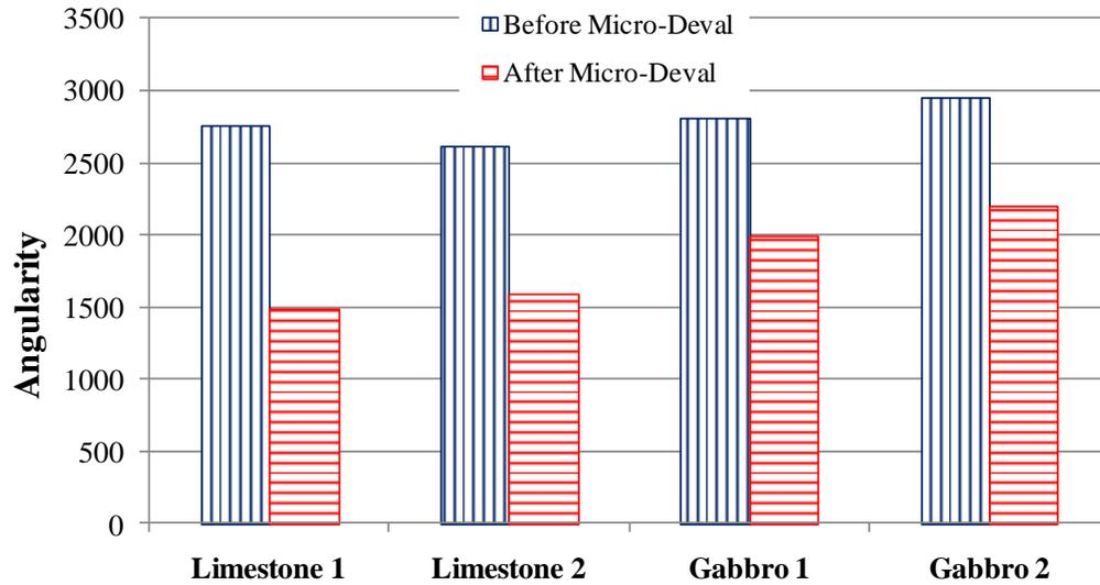
**Figure 3.7** Average angularity index before and after the micro-deval test (Masad et al. 2011)
