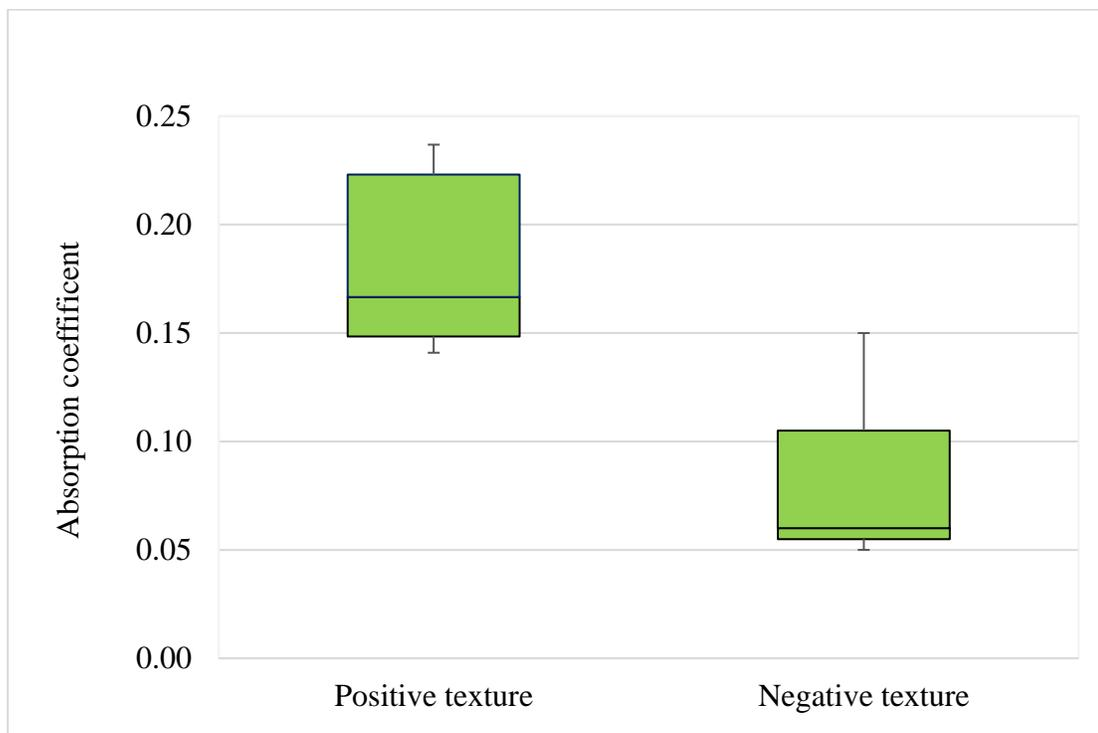
**Figure 4.39** Absorption coefficient of asphalt samples for positive and negative texture
