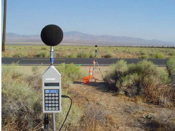
**Figure 2.3** SPB measurement apparatus (Rochat et al. 2010)
