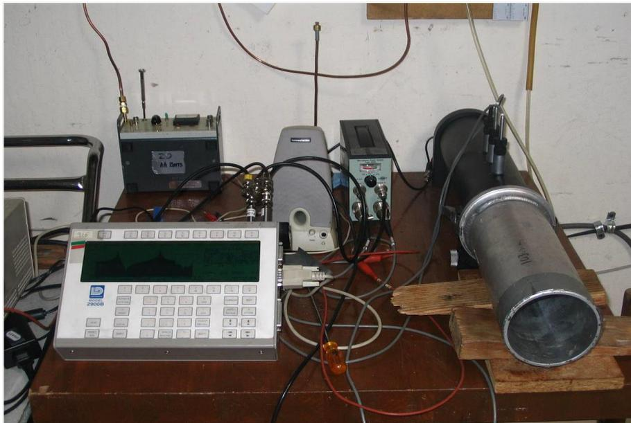
**Figure 2.13** Impedance tube system (Ongel et al. 2007)
