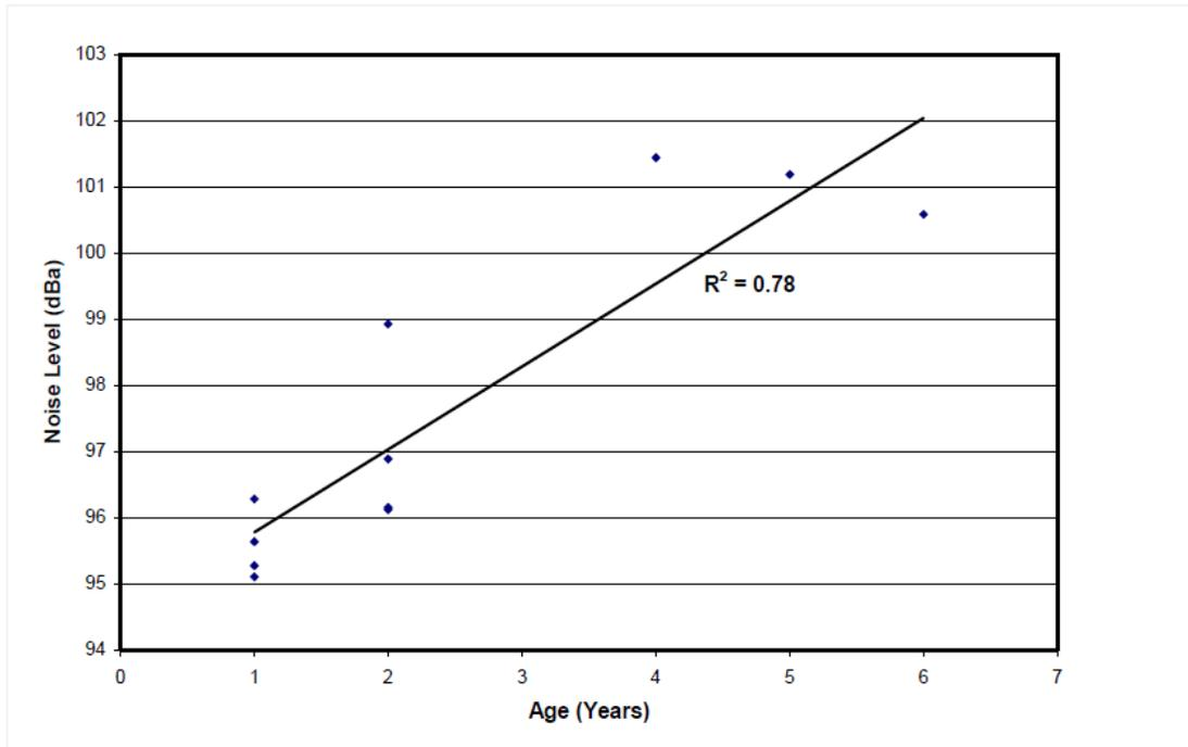
**Figure 2.18** Effect of Age of Pavement on Noise (Hanson et al.2004).
