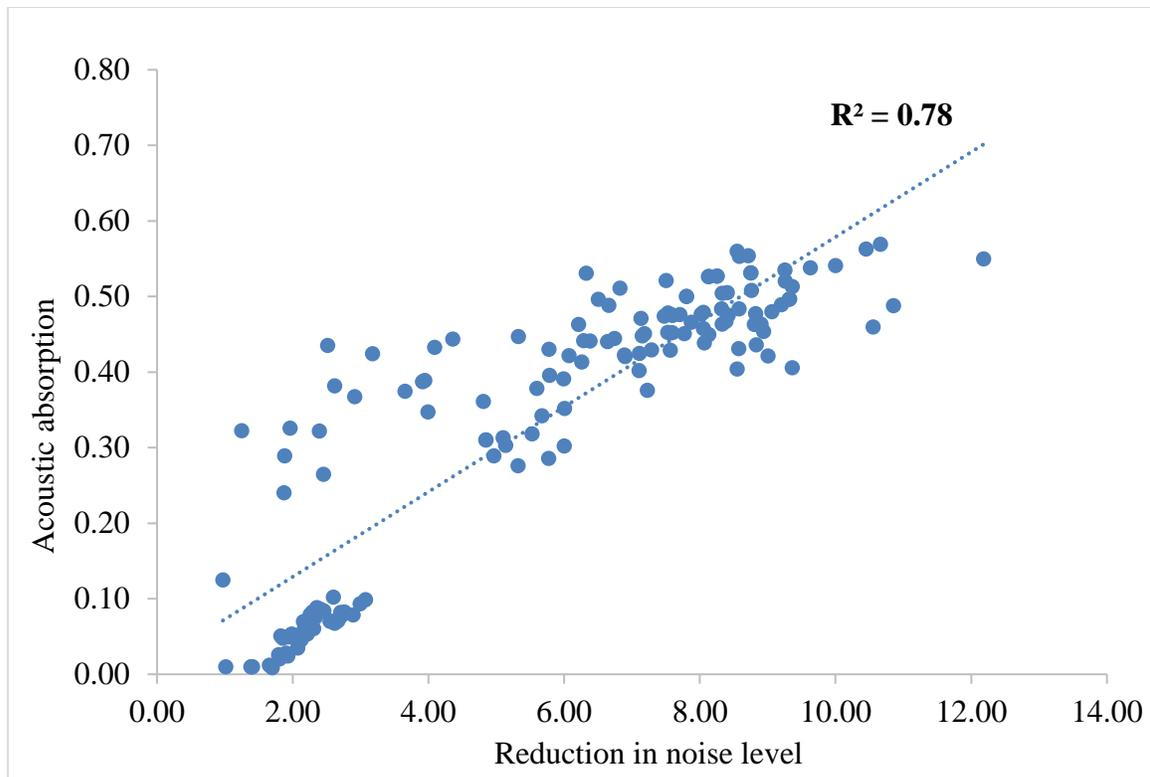
**Figure 4.27** Correlation between absorption coefficient and noise reduction level
