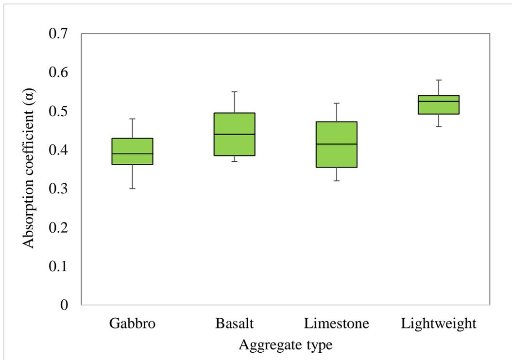
**Figure 4.20** Box plot of acoustic absorption of pavement for different types of aggregate
