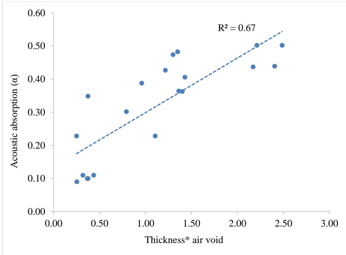
**Figure 4.14** Correlation between acoustic absorption of pavement and thickness x air void (Gabbro)
