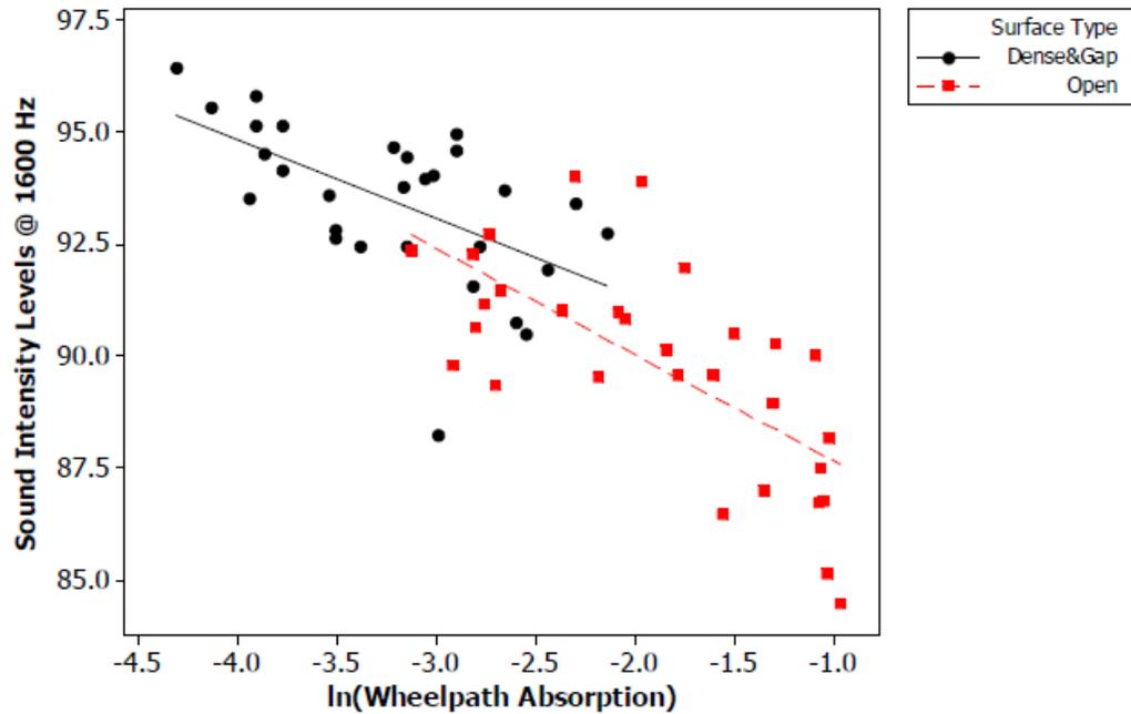
**Figure 2.12** Sound intensity levels at 1,600 Hz versus the absorption values.
