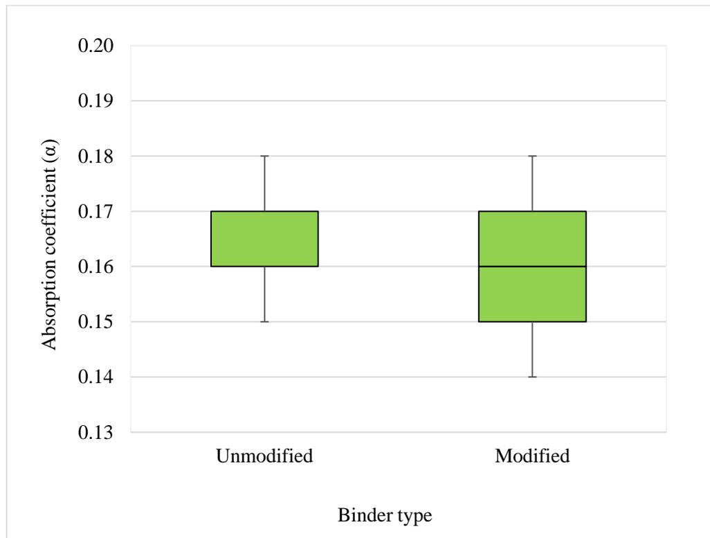
**Figure 4.21** Box plot of acoustic absorption of pavement for modified and unmodified binder.
