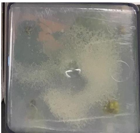
Image 3.4. Bottom view of a tissue culture vessel containing SNRF medium with constituent precipitate(s) from preliminary SNRF formulations. The abbreviation SNRF stands for sap-based nutrient ratio formulation.
