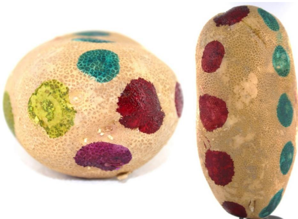
Figure 2-1. Predetermined impact locations on each tuber for trial three. Twenty locations were impacted on each tuber: each of the four sides (both flat surfaces and shoulders) were marked in five spots (bud, mid-bud, middle, mid-stem, stem) that created a longitudinal line from the bud end to the stem end of the tuber.
