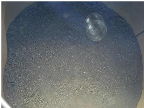
Figure 3.12. Ternary salt used in the molten salt dissolution of used nuclear oxide fuels.
