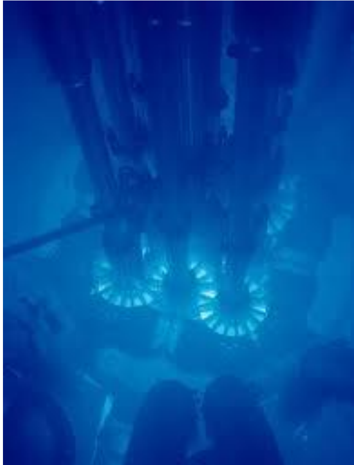
Figure 1.4. Core of Advanced Test Reactor with a characteristic blue Cherenkov radiation.
