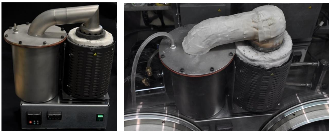
Figure 5.1. Furnace and off-gas trap assembly before (left) and after (right) installation in glovebox.
