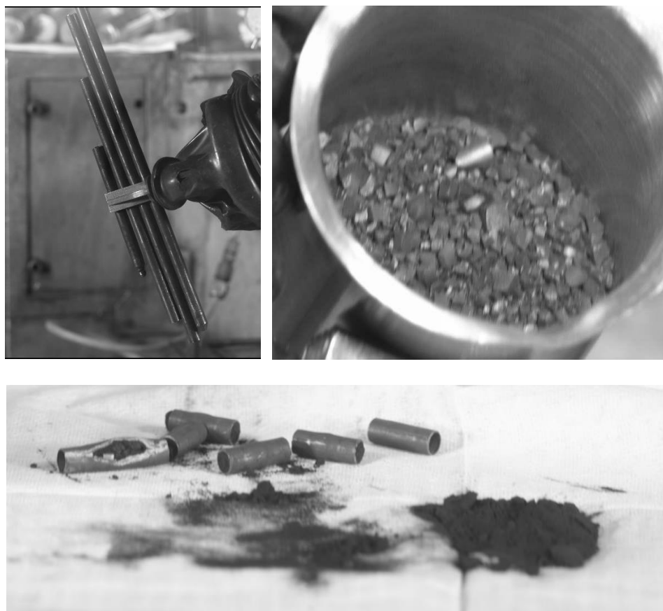
Figure 3.9. Cut (upper left) and declad BR3 fuel element by crushing (upper right) and by DEOX process (bottom).
