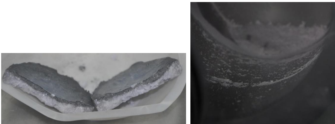
Figure 5.6. Bottoms (left) and distillate (right) products from run 1.
