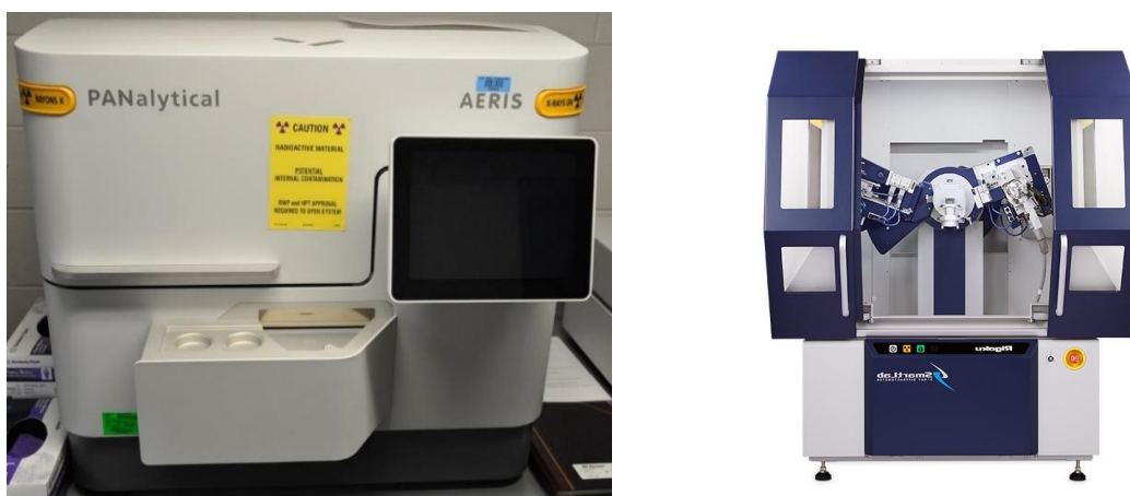
Figure 3.18. PANalytical X-ray diffractometer in FASB (left) and Rigaku X-ray diffractometer in CAES (right).
