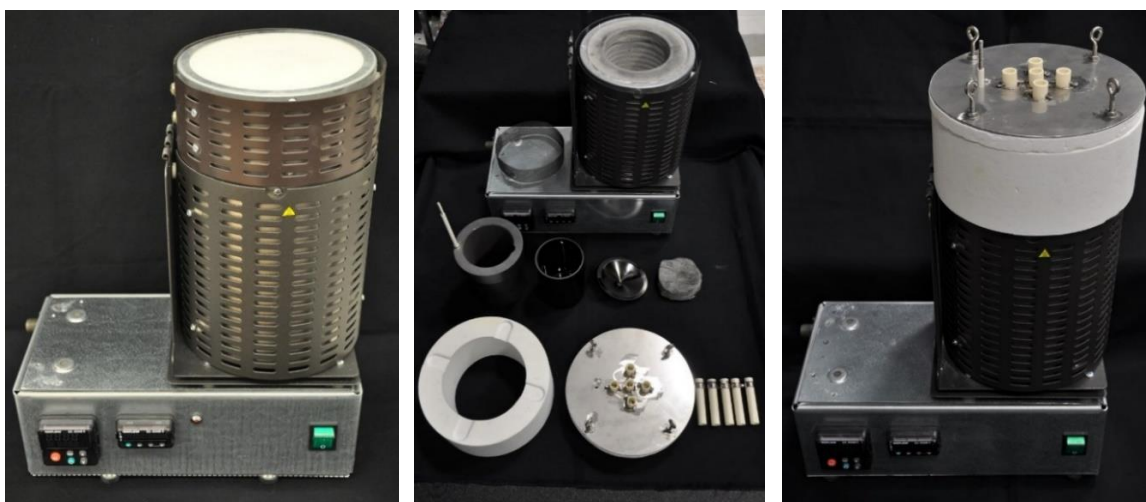
Figure 7.1. Furnace and components for synthesis runs, including heat-up configuration (left), disassembled components (center), and electrolytic cell configuration (right).
