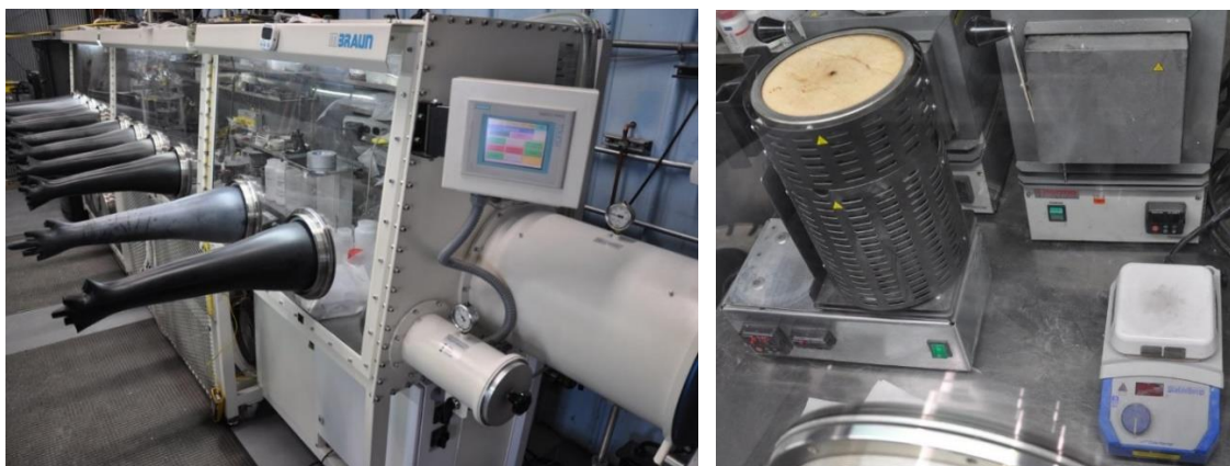
Figure 3.7. Non-radiological glovebox (left) in EDL and installed equipment (right).
