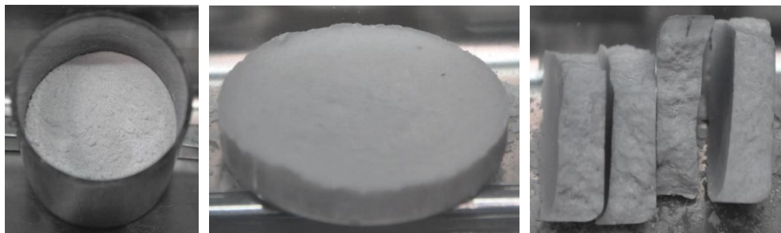
Figure 5.7. Waste-form blend before (left) and after (center) consolidation and breaking (right).
