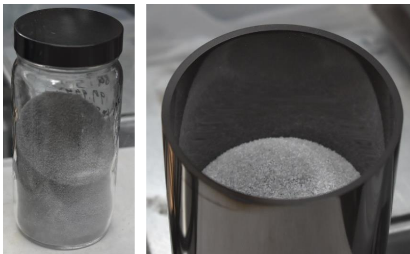
Figure 7.4. Uranium metal powder, ammonium chloride, and lithium chloride – potassium chloride blend before (left) and after (right) loading in glassy carbon crucible.
