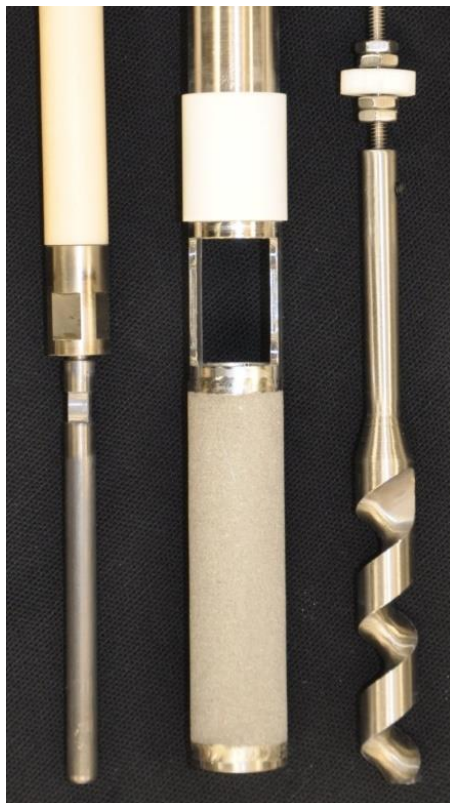
Figure 4.8. Tantalum rod (left) and sintered stainless-steel tipped basket assembly (center and right) for oxide fuel loading in chemical-seed dissolution study.
