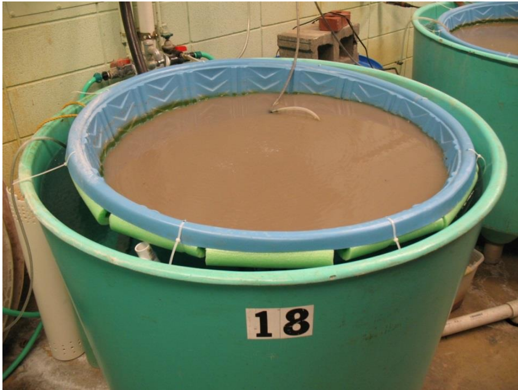
Figure 2.3 – Temperature controlled set-up used to culture of Lepidurus lemmoni in the laboratory common garden study. A 120 cm plastic wading pool was floated in a 1000 L fiberglass tank through which temperature-controlled water was passed to maintain a constant water temperature. Gentle aeration was provided via an airstone. Turbidity resulted from the suspension of very fine sediment particles when the sediments were wetted, and are reflective of conditions in the native lake habitats which were simulated in this experiment
