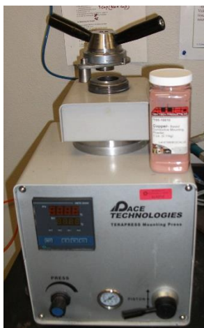
Figure 3.12 TERAPRESS™ TP-7001 compression mounting press.
