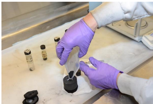
Figure 3.7 Loading I-85 graphite dies for SPS.
