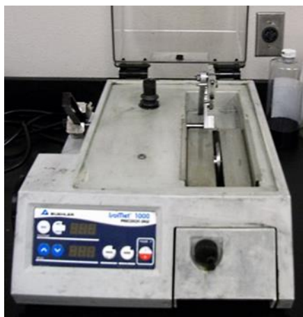
Figure 3.10 IsoMet™ 1000 precision sectioning saw.
