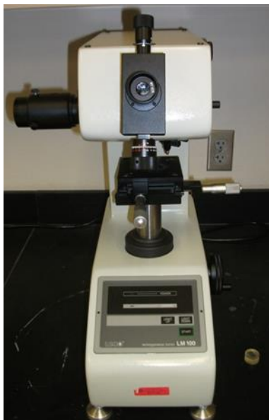
Figure 3.16 LECO LM100 micro-indentation hardness machine.
