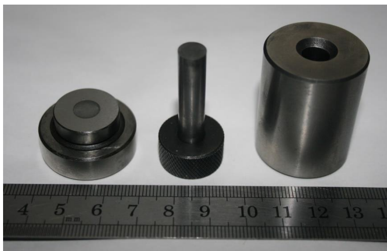
Figure 3.2 Die and punch assembly.
