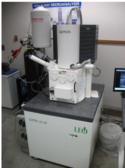
Figure 3.13 Field Emission Scanning Electron Microscope, LEO Supra 35VP.
