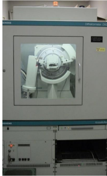
Figure 3.14 Seimens D5000 powder X-ray diffractometer.
