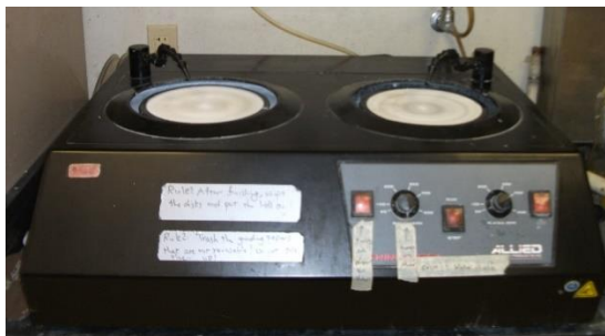
Figure 3.8 TwinPrep 3™ polishing machine.
