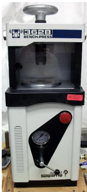
Figure 3.1 BenchPress™ 3628 pneumatic press
