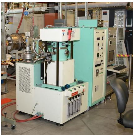
Figure 3.5 Dr. Sinter SPS-515S. Located at CAES, Idaho Falls, ID.
