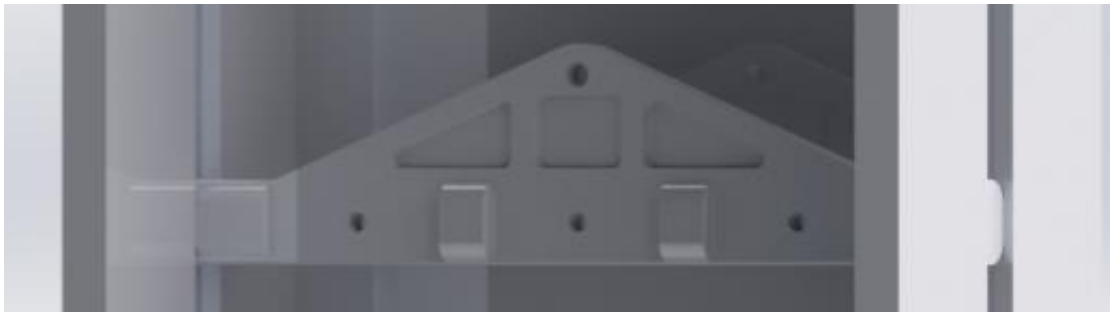
Figure 3.6. Spring/cable attachment for force transmission. Designed to transmit the force from 6 individual spools to a cable that can be routed through PRISM.
