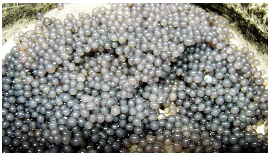
Figure 2.4: Sodium Alginate beads with encapsulated KB-1
