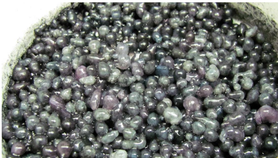
Figure 2.5: PVA/SA beads with encapsulated KB-1
