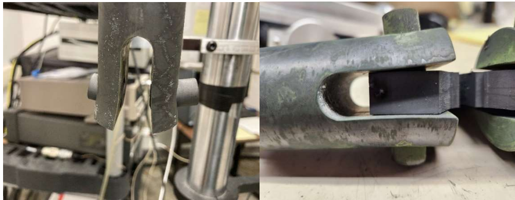
Figure 17: Inconel 718 sheared pin and deformed grips on FCG and CCG frames.
