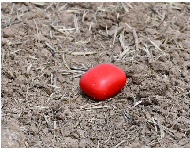
Figure 4.4: Example of an instrumented sphere [Techmark, Inc. Impact Recoding device (IRD) TM ] placed on top of soil to be harvested with potatoes to monitor the impacts during harvest. Courtesy of Rabecka Hendricks.
