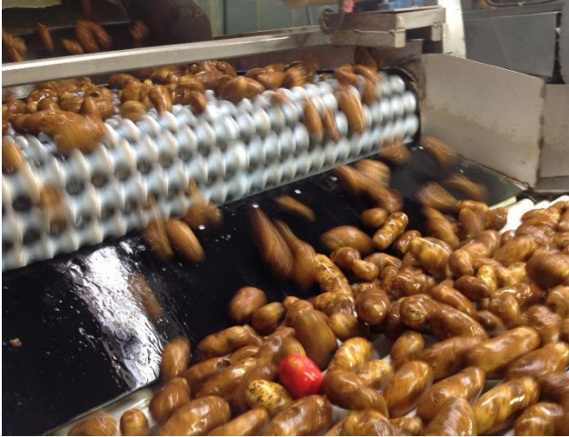
Figure 4.5: An IRD™ (red ball) recording impacts as potatoes are being conveyed in a fresh pack operation. Courtesy of Carlos Centeno
