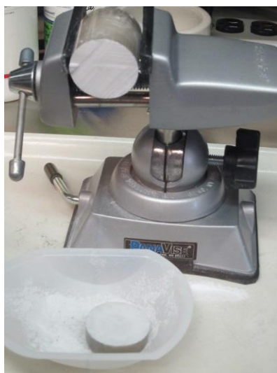
Figure 3.12 The bottom of the LiCl-KCl ingot is cut off as part of a method to ensure \text{ZrCl}_4 is dissolved into the eutectic.
