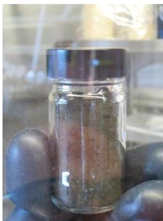
Figure 3.4 75 wt% \text{UCl}_3 in LiCl-KCl eutectic used in the experiments provided by INL.
