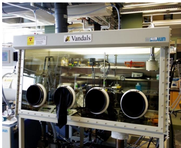
Figure 3.1 MBraun argon atmosphere glovebox in which all uranium experiments were conducted.
