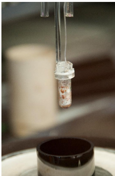
Figure 3.9 5.0 mol% Ag/AgCl reference electrode in a Pyrex® body used in the electrochemical experiments.
