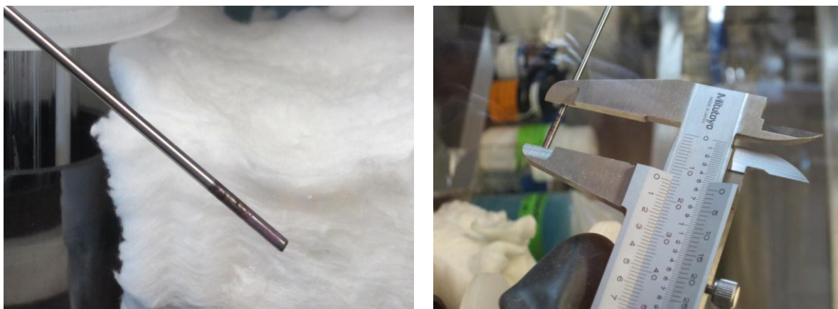
Figure 3.20 Example of working electrode immersion depth measurement from 1.00 wt% \text{UCl}_3 in \text{LiCl-KCl} at 773 K.
