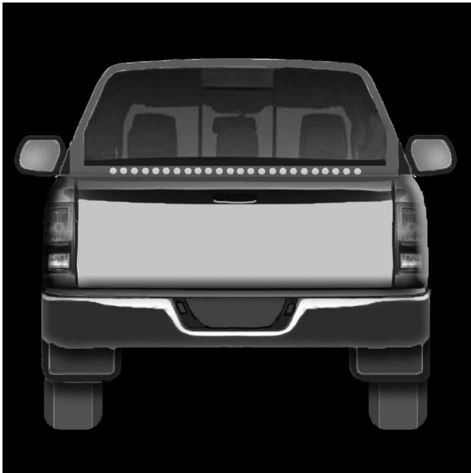
Figure 3. Rear view of truck with array of unlit deceleration display lights.
