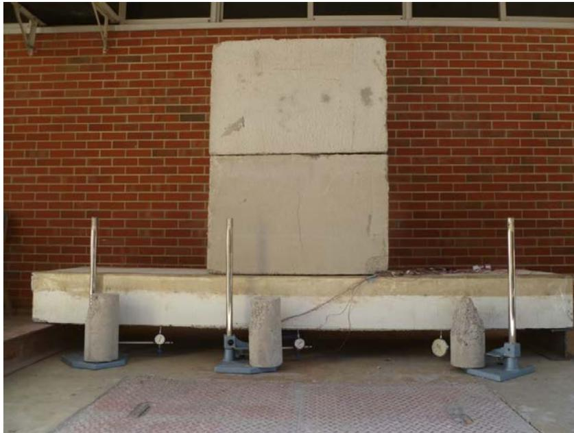
Figure 121 – Creep test set up for 10" FPCS panel
