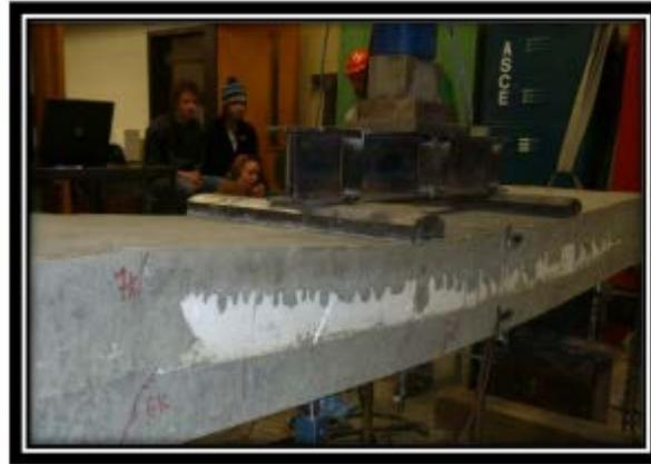
Figure 43 – Actual four-point bending test
