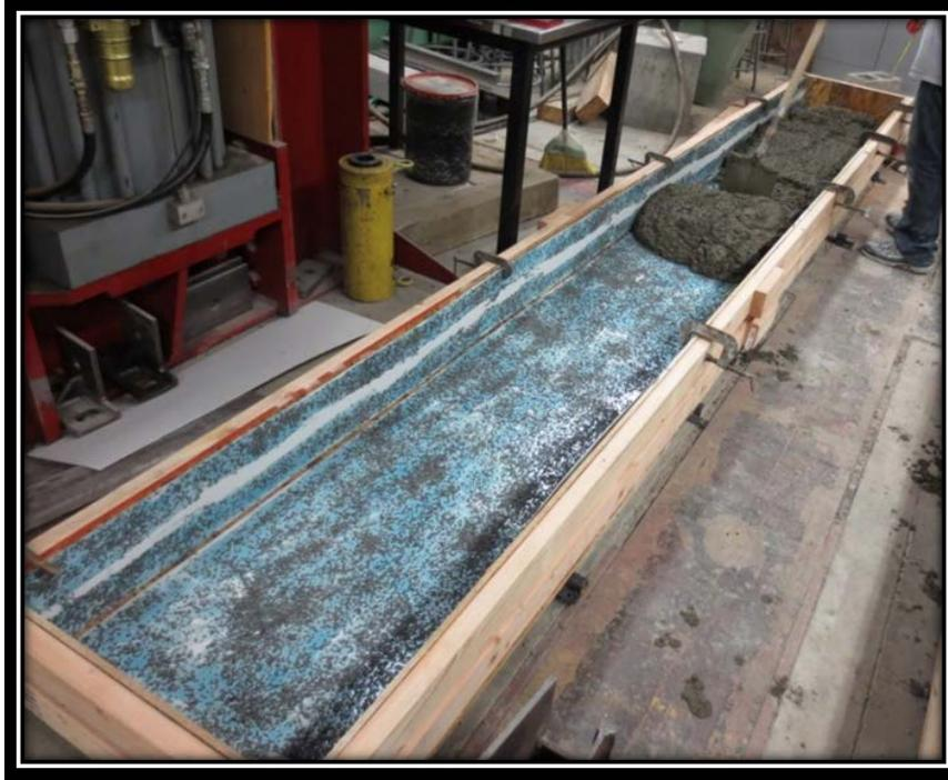
**Figure 66 – Full scale FPCS first concrete lift pour<sup>[44]</sup>**
