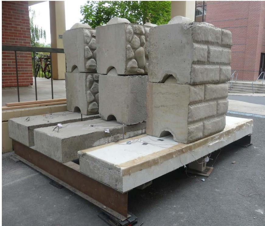
**Figure 122 – Creep test panel set up for 8'' FPCS, 10'' sandwich and 10'' solid panel**
