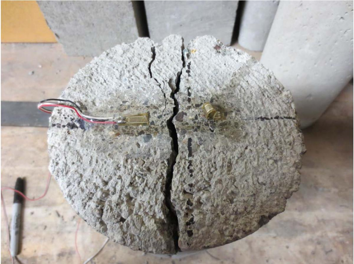
**Figure 54 – Splitting tensile test specimen**
