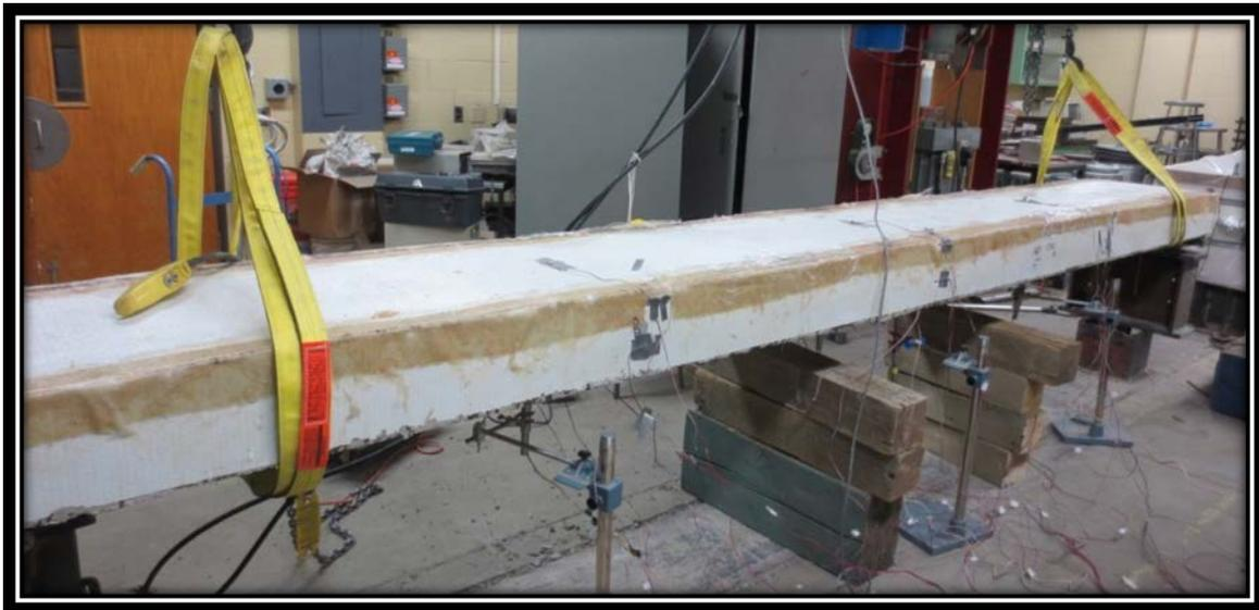
**Figure 69 – Full-scale FPCS panel in testing apparatus<sup>[44]</sup>**
