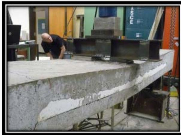
Figure 45 – Actual three-point bending test
