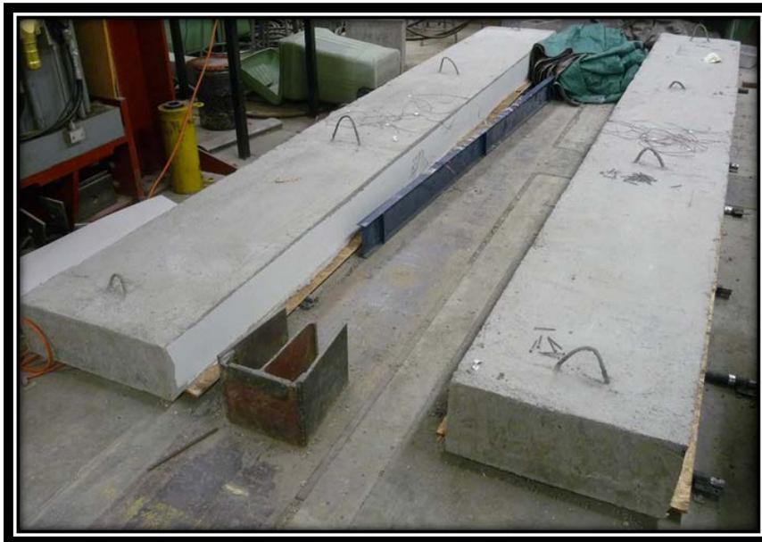
**Figure 67 – Cured and stripped full-scale FPCS specimens<sup>[44]</sup>**
