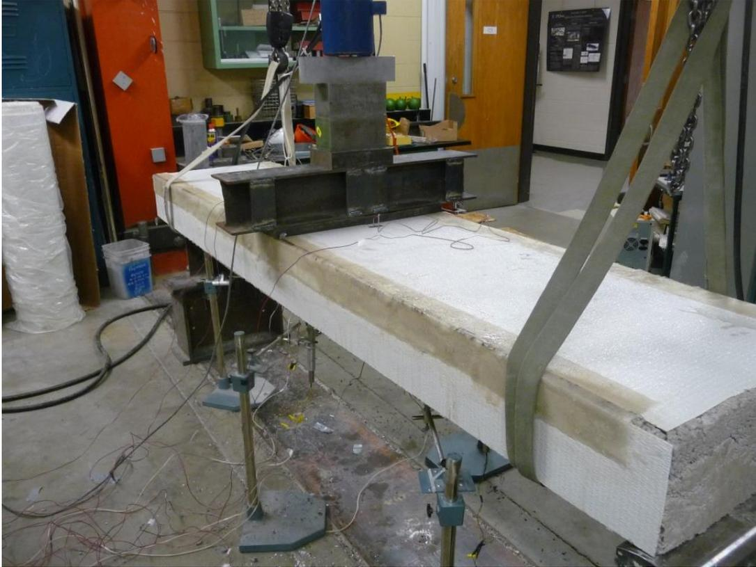
**Figure 58 – 10 in. FRP sandwich panel (108SEGDN10L3PTFFPCSS1) in testing apparatus**
