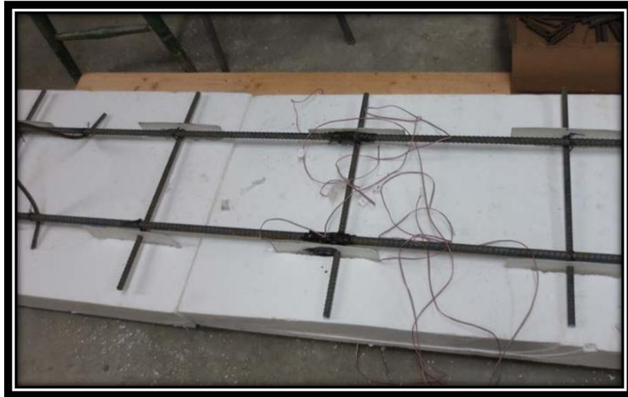
**Figure 65 – Full scale FPCS panel insulation, rebar and strain gages<sup>[44]</sup>**
