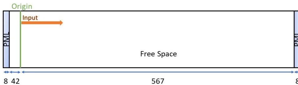
Figure 3.4: Simulation space of 625 cells with free space and the PML. The input travels from the origin to the right.
