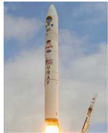
Figure 4: Minotaur IV chemical rocket [48]
