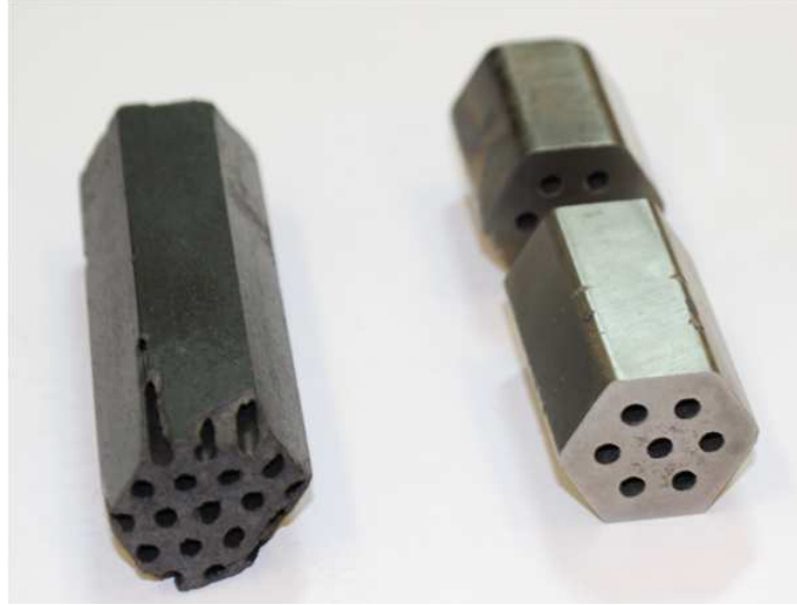
Figure 6: Graphite NERVA fuel element (left) and new, tungsten based fuel element (right). Image courtesy of the Center for Space Nuclear Research
