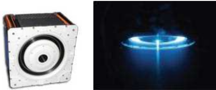
Figure 8: Hall Effect thruster image (left) and while operating (right) [23]
