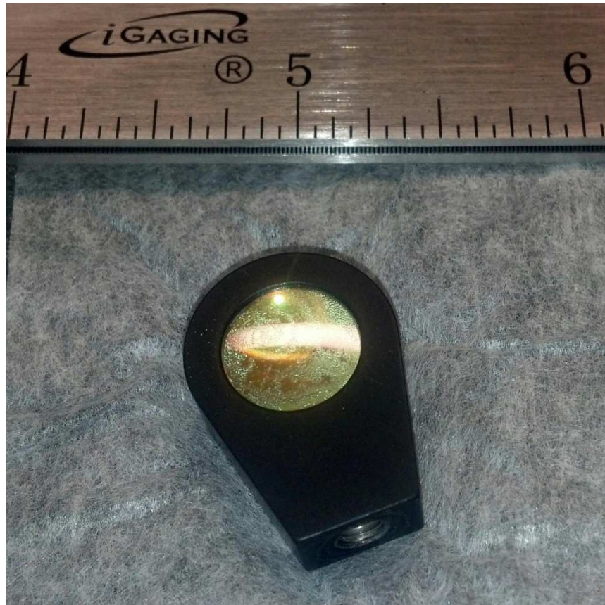
Figure 17: Focusing lens damaged by laser
