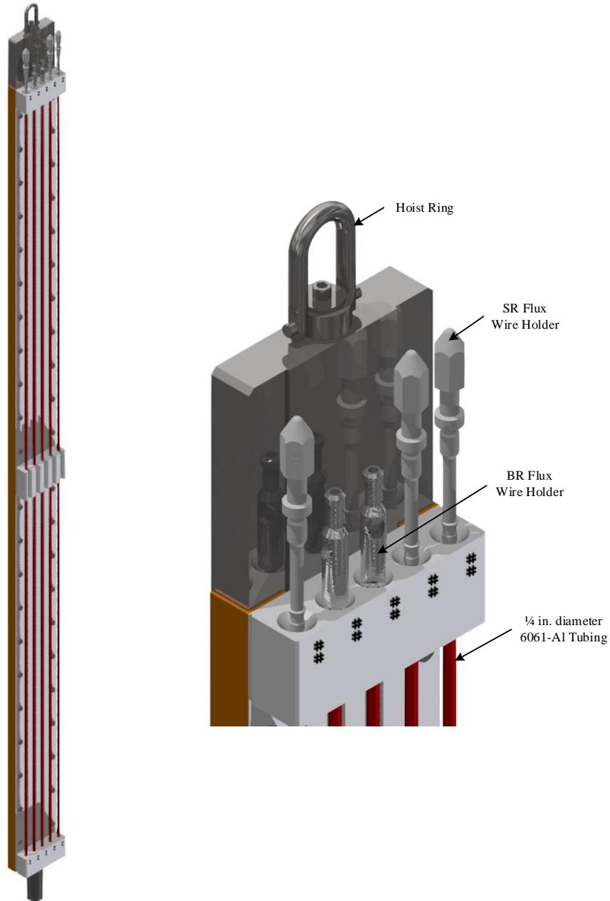
*Figure 4.5: Flux wire holder magazine*
