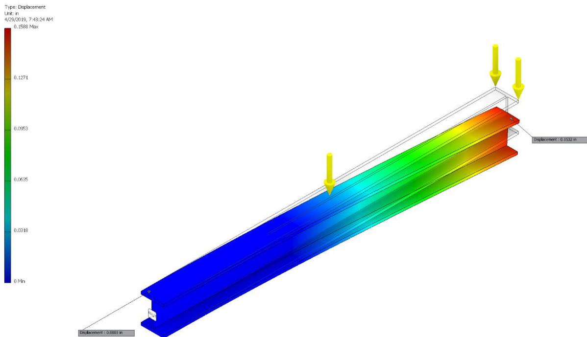
Figure E3: FEA Results - Displacement of cantilever beam due to distributed and point loads.
