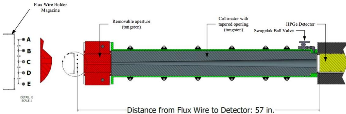
**Figure 4.6: Gamma detector and flux wire holder magazine scanning configuration**
