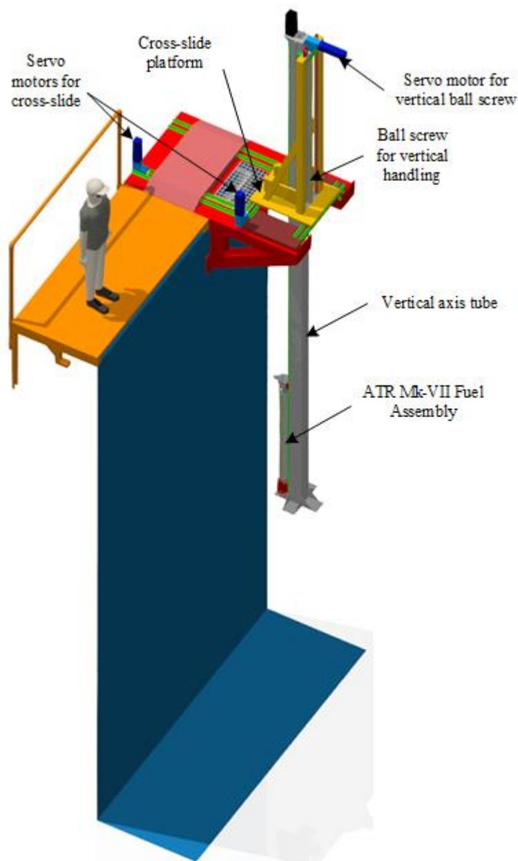
*Figure 3.1: ANDES handling system concept*
