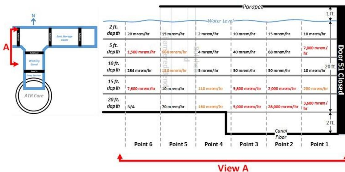
Figure 4.2: ATR working canal underwater survey (Survey-M-20180315-15)
