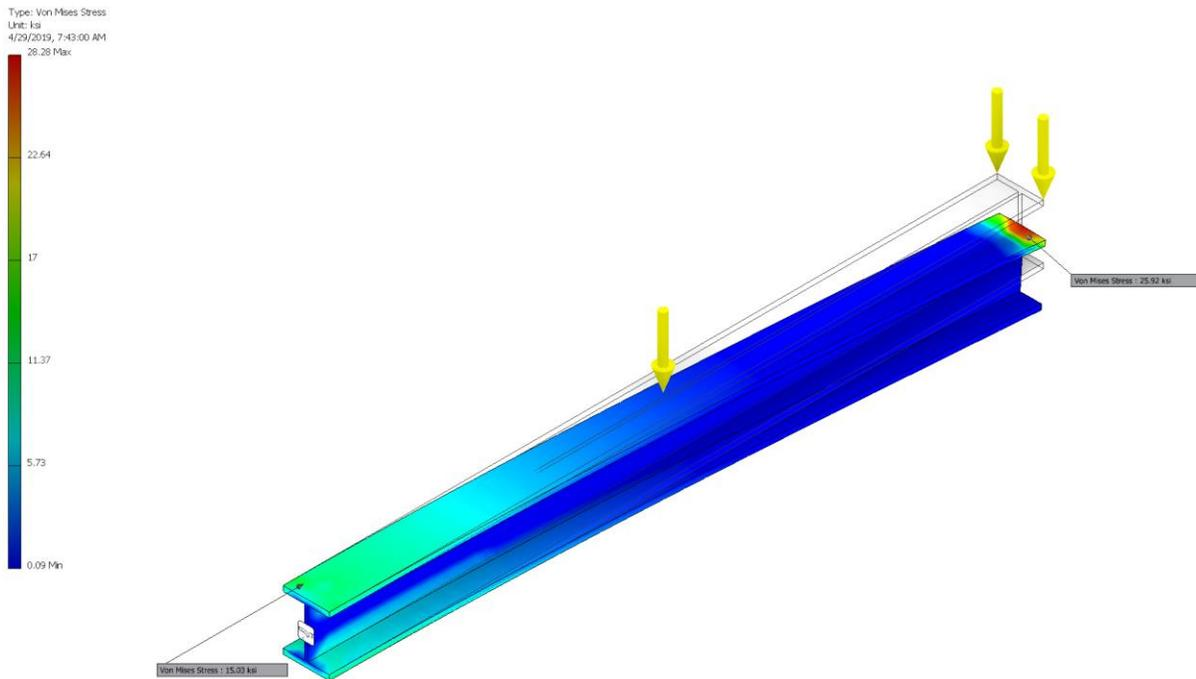
*Figure E1: FEA Results - von Mises stress of cantilever I-beam with total range of observed stresses.*
