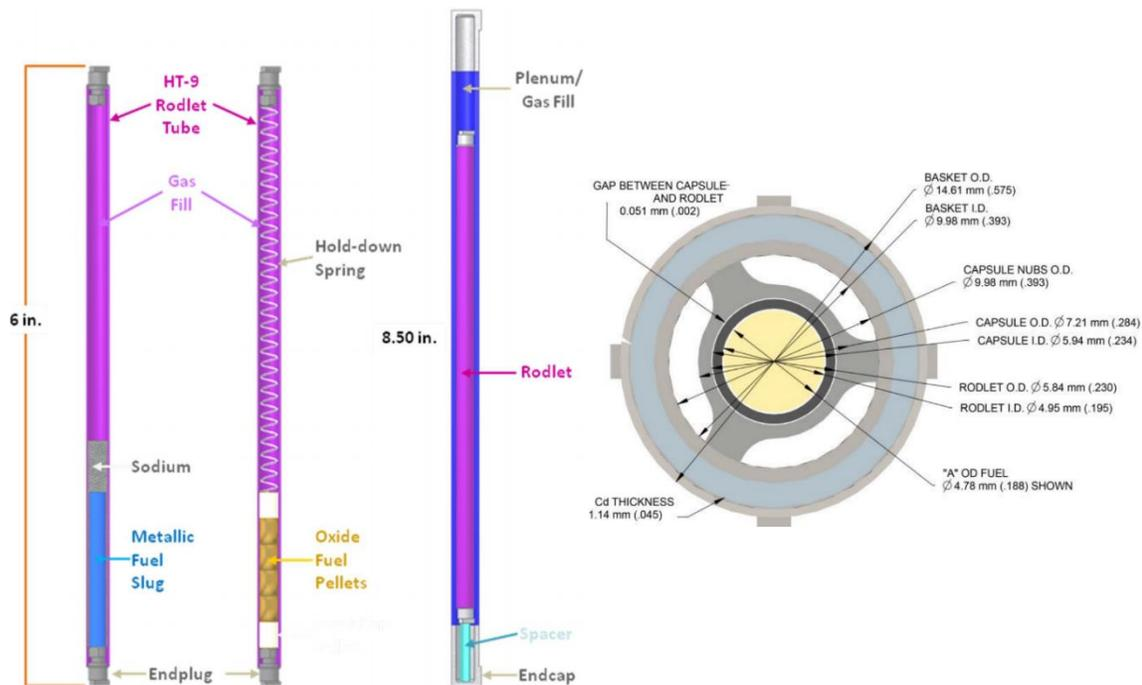
*Figure 2.3: AFC-4 rodlet assembly and inner test train assembly (left); Cross-section of AFC-4 capsule contained in cadmium-lined experiment basket (right)<sup>25</sup>*
