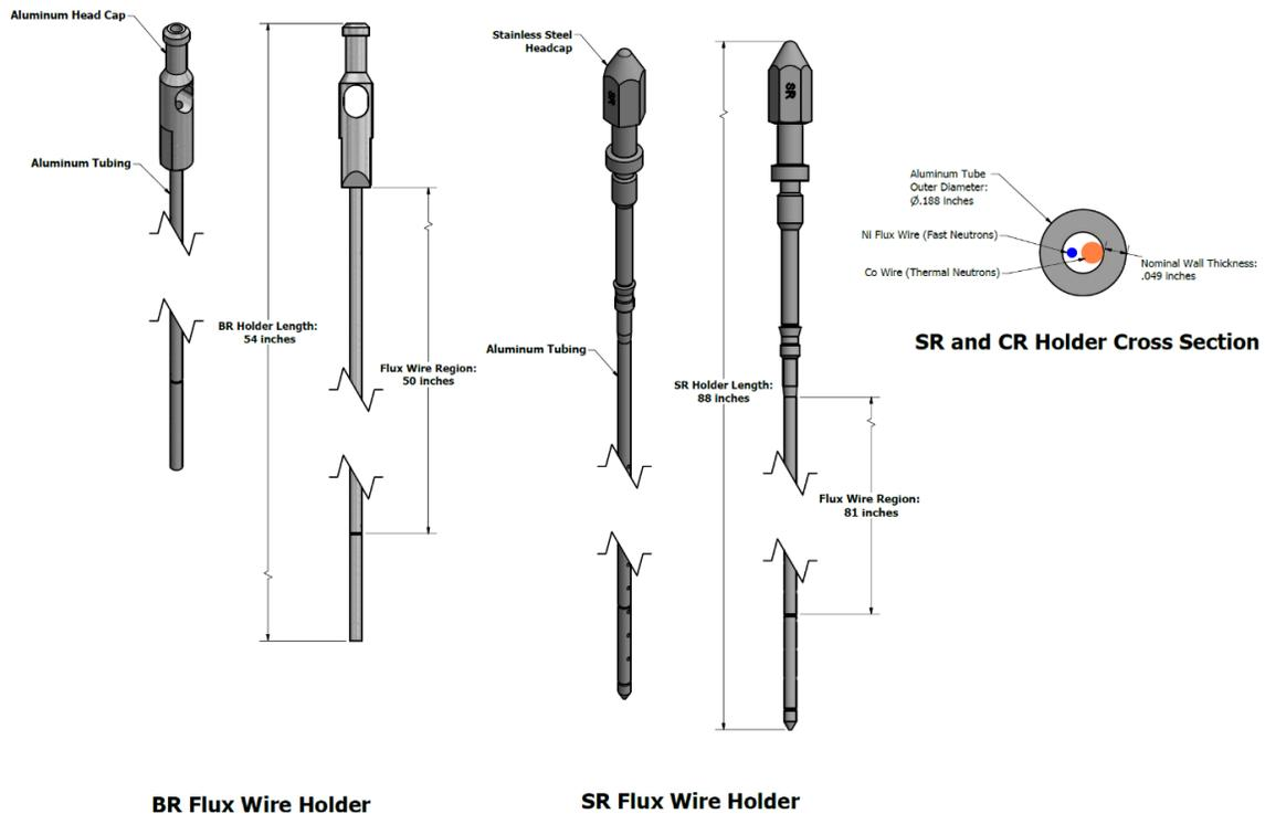
Figure 2.2: BR flux wire holder (left) and SR flux wire holder (middle); Cross-section with flux wires (right)
