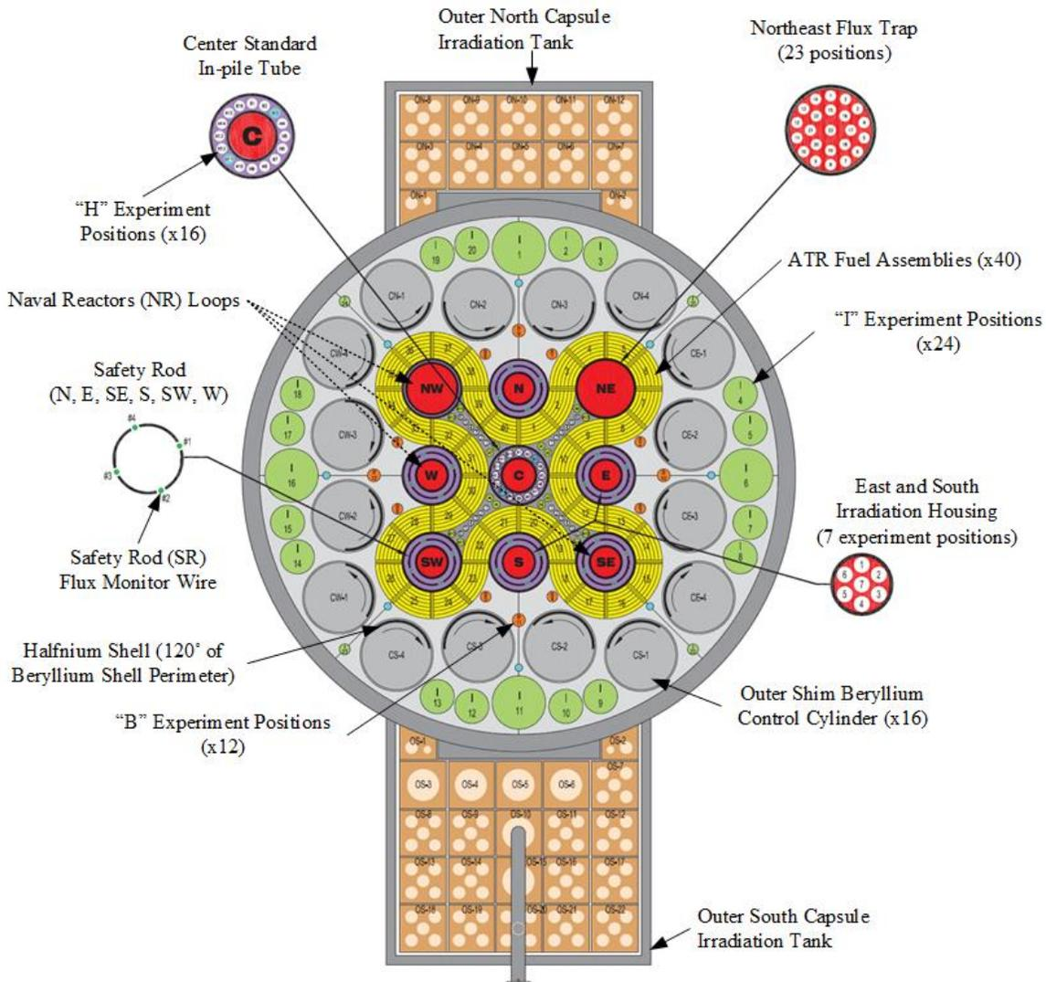
Figure 1.1: Cross-section of Advanced Test Reactor core<sup>10</sup>
