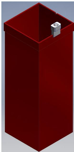
*Figure 3.7: ANDES passive coolant container with source holder*
