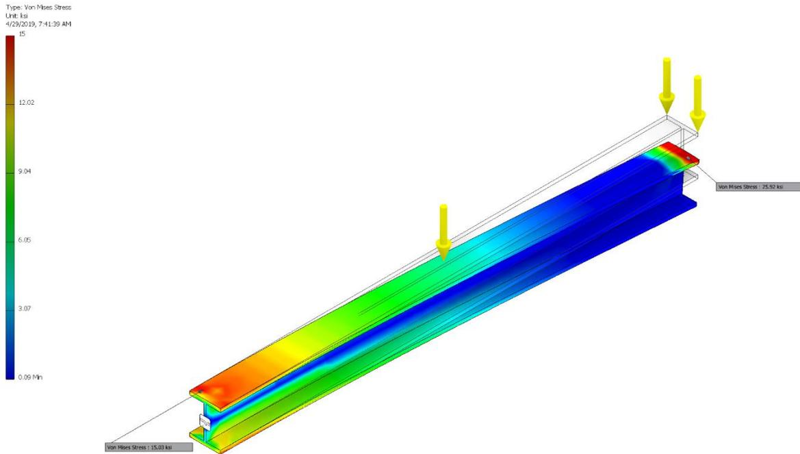
Figure E2: FEA Results - von Mises stress of cantilever I-beam with narrowed range of stresses.
