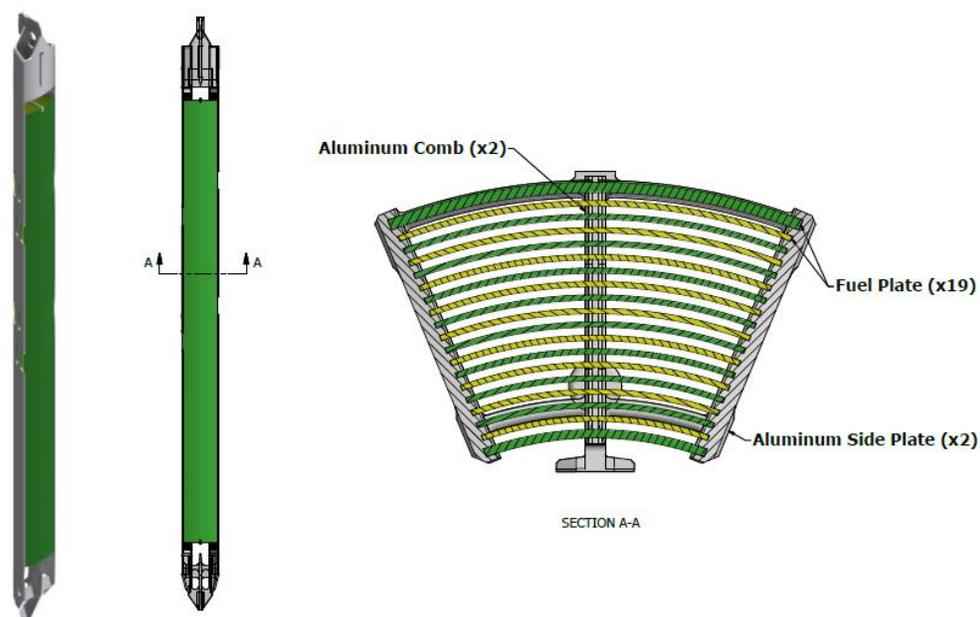
*Figure 2.1: Isometric view of Mark-VII fuel assembly (left); Cross-section schematic of Mark-VII fuel assembly (right)*
