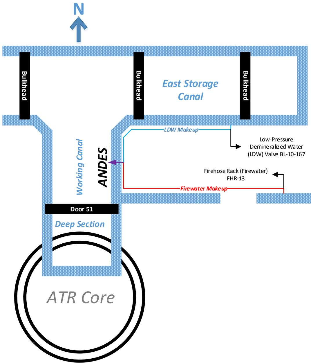
Figure 3.8: Fire water and LDW connections<sup>55-56</sup>
