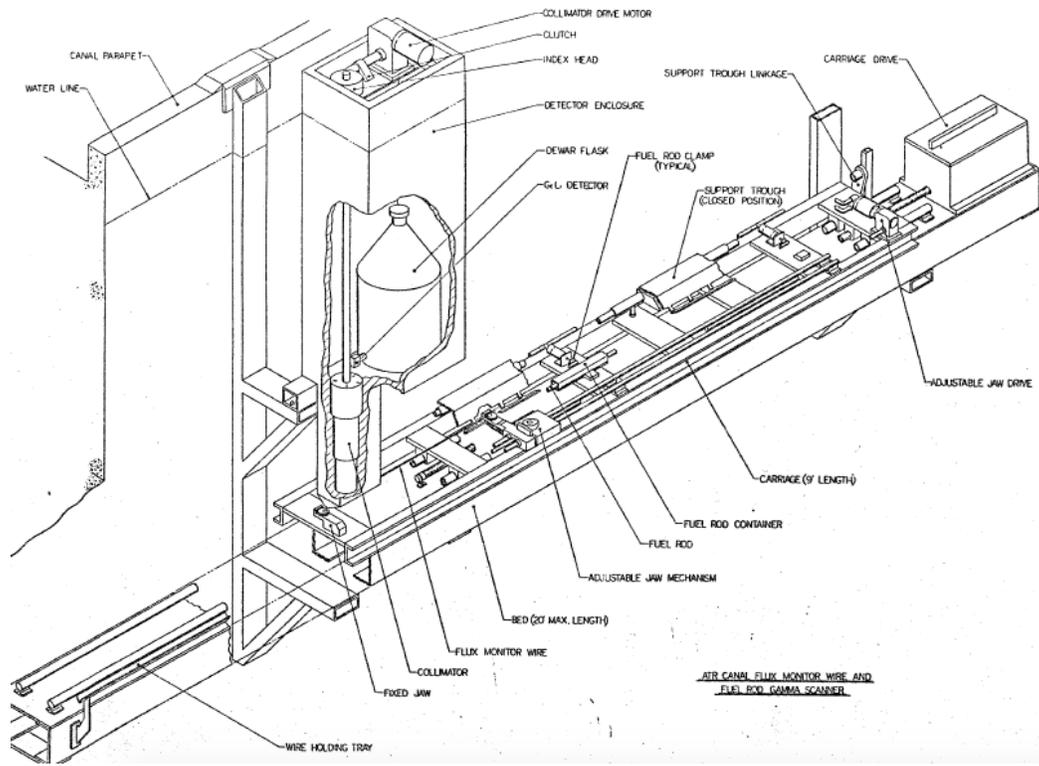
Figure 1.2: 1978 Conceptual design of an ATR canal high-resolution flux wire monitor and fuel rod gamma scanner<sup>15</sup>
