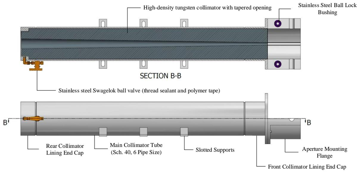
Figure 4.3: Collimator weldment
