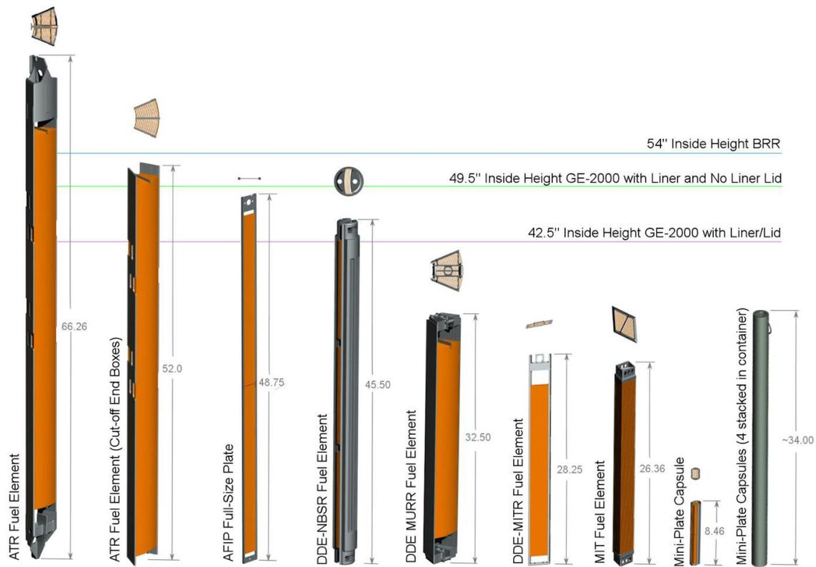
Figure 2.5: Plate-type experiment overview<sup>26</sup>
