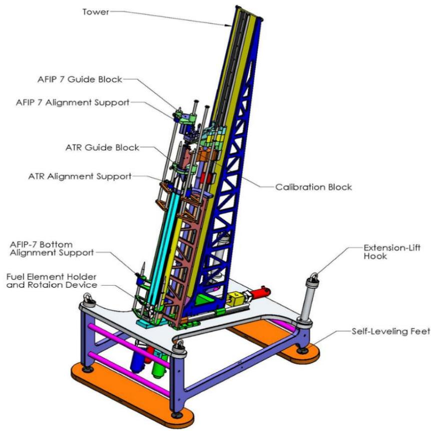
Figure 1.3: AFIP channel gap probe
