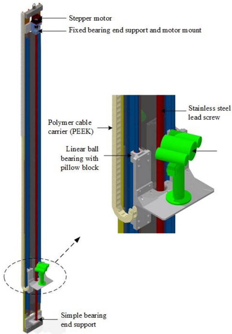
*Figure 3.3: ANDES camera handling system*
