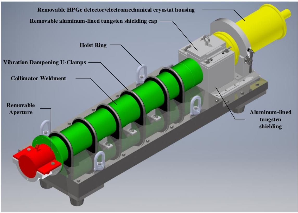
Figure 4.4: Sealed collimator (green), removable aperture (red) and removable detector/cryostat housing (yellow) mounted onto support frame tray
