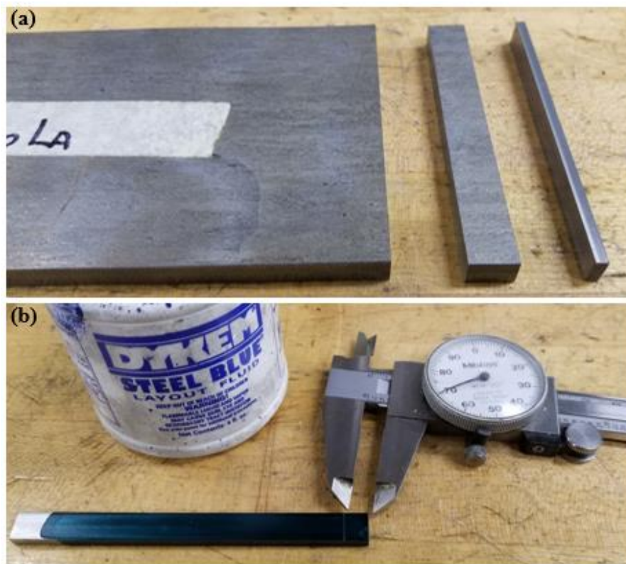
Figure 2.3: Coupon preparation from AR plate: (a) Plate of Mo-La, cut then milled (b) width measured and scored on steel blue layout fluid for additional cut, then milled.
