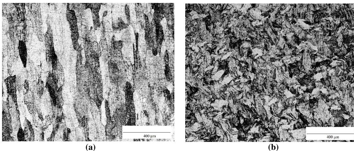
Figure 3.1: As-received microstructure of molybdenum rod (a) longitudinal (b) transverse sections.
