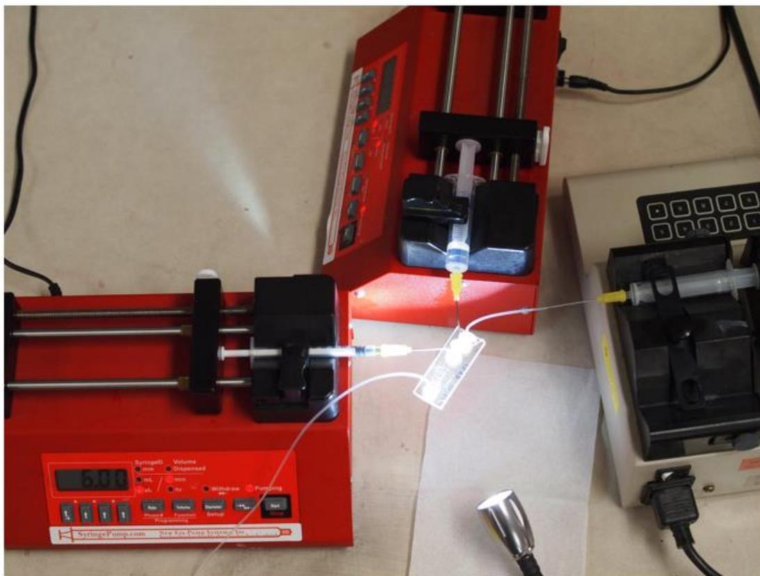
Figure 4.S4. Photograph of particle generation chip in operation. Left syringe contains the aqueous phase; top syringe contains the oil phase; right syringe contains the initiator solution.
