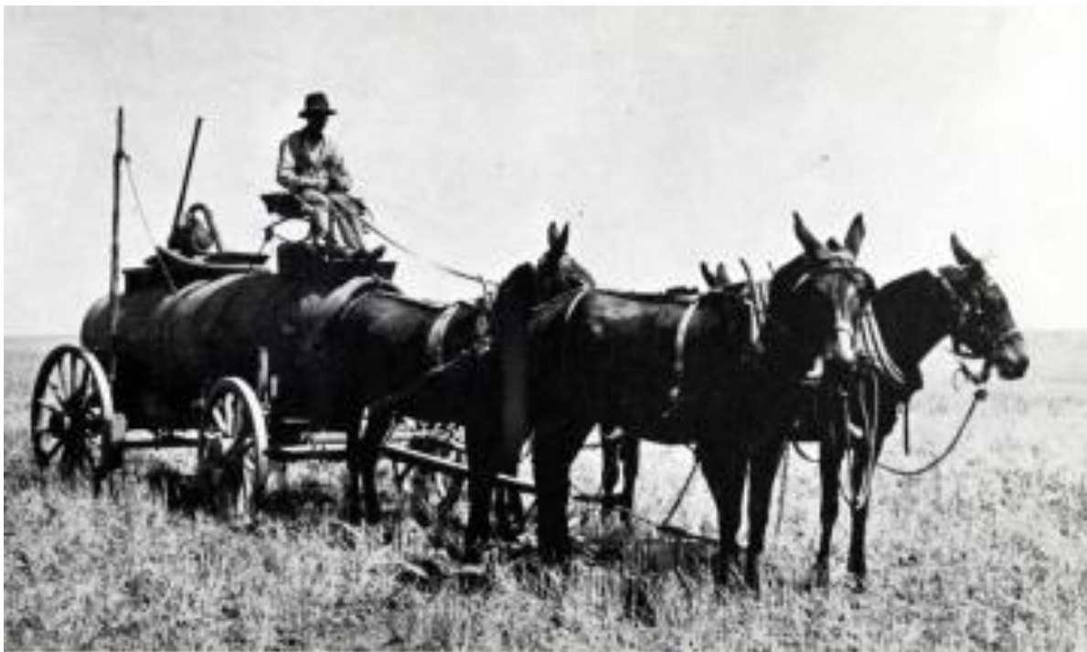
Figure 10: Four Mules on a Typical Water Wagon. With a man-powered water pump on the top of water tank. Tall stick with the rope is attached to the wagon is the brake, 1900. 328
