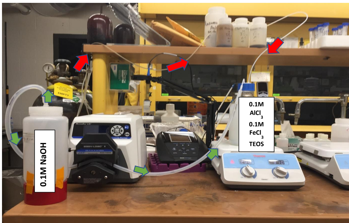
Figure 3.1. Annotated picture of allophane synthesis set up. NaOH is titrated through tube in direction of green arrows. Red arrows indicate flow of nitrogen in Fe(II) syntheses.
