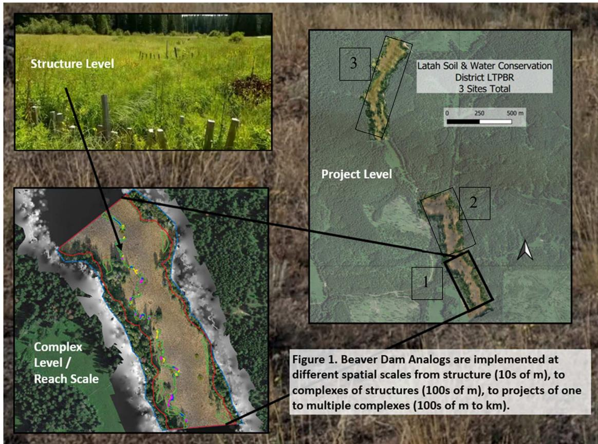
Figure 1. Beaver Dam Analogs are implemented at different spatial scales from the structure, complex, to project scales.
