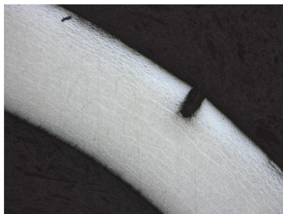
Figure 5-10. Metallographic image of a cladding tube with 412 ppm hydrogen after pressure testing at 400 °C.
