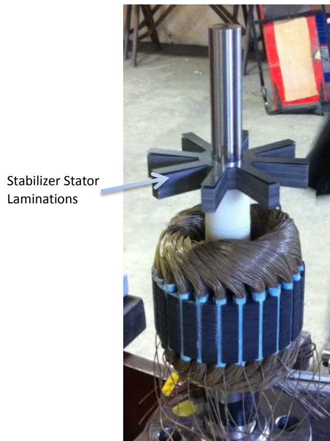
Figure 1.5: Stabilizing laminations and wrapped FRRM laminations
