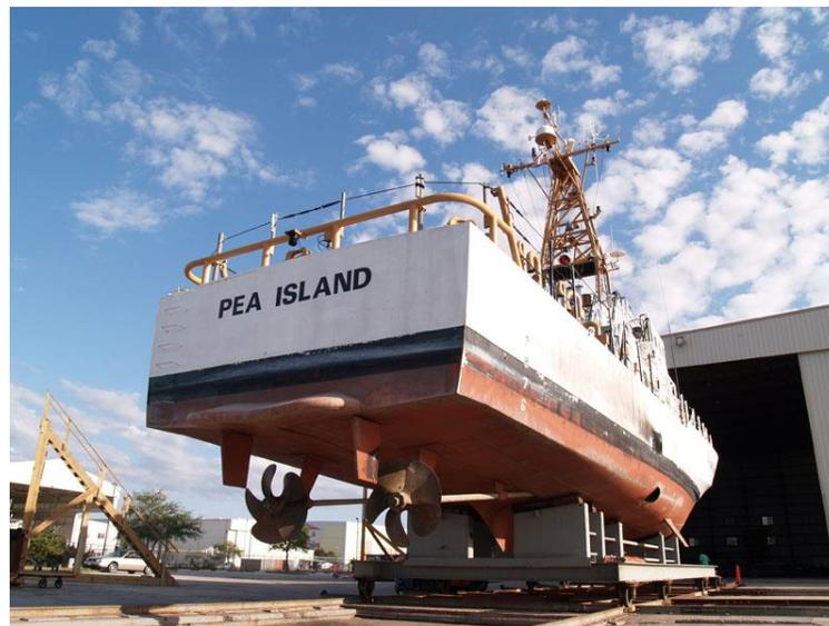
**Figure 3: A typical twin screw set up.**
