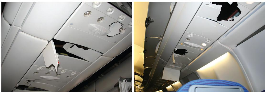
FIGURE 1.1: Photographs of the damaged Airbus after the SEU [5].
