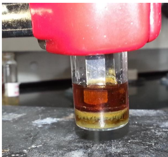
Figure 14 Sodium Chloride Electrolysis Reaction with Chloroform
