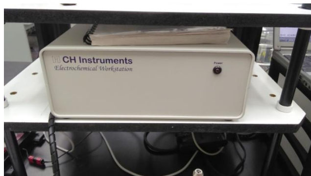
Figure 3.6: CHI 760B potentiostat used for all electrochemical experiments.
