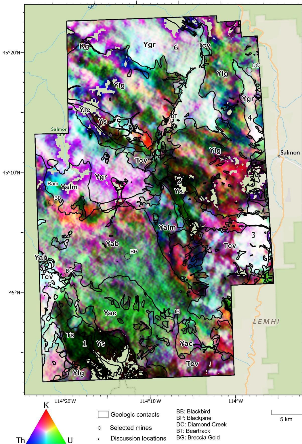
Figure 3.6 RGB color composite image of airborne gamma radiation measured concentrations of potassium, uranium, and thorium within the study area.
