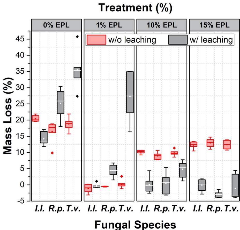
Figure 21. The mass loss percentage of three fungi performed at 1%, 10%, 15% and control (water treated) treatments.
