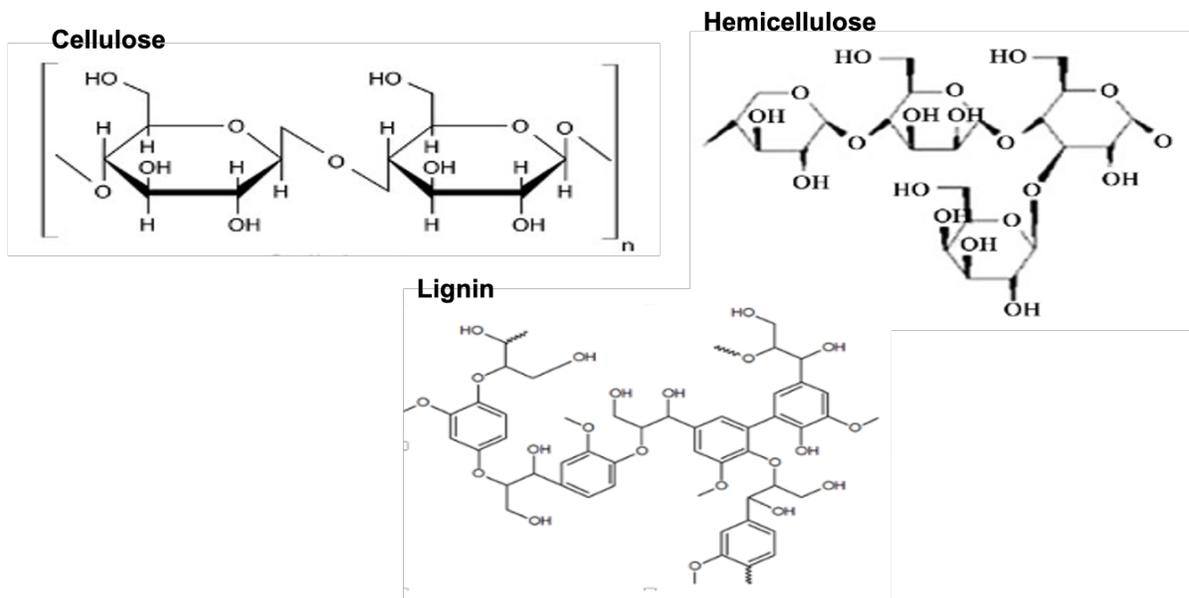
Figure 1. The chemical structure of cellulose, hemicellulose, and lignin (Muktham, et al., 2016).
