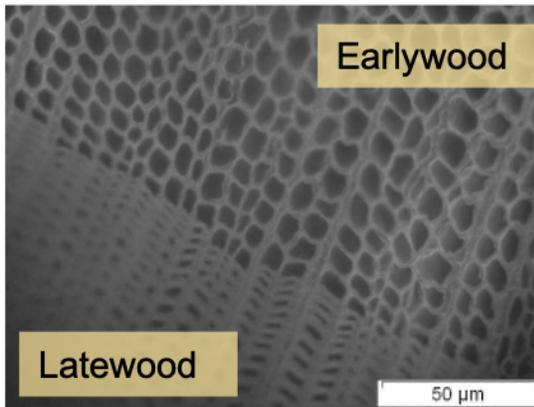
Figure 3. The cross-section of tracheids in softwood (southern pine, *Pinus taeda* L.).
