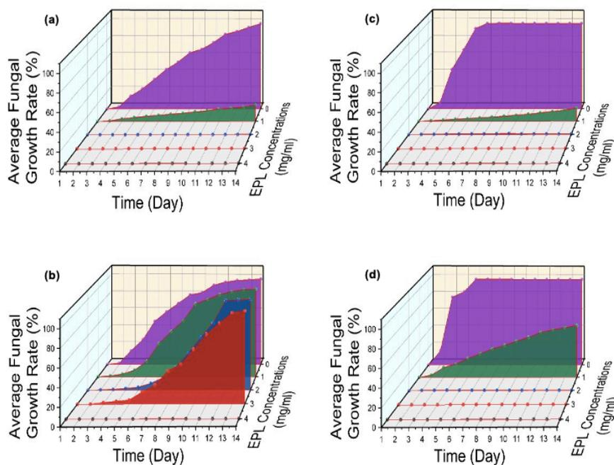
Figure 10. The average fungal growth rates of two brown rot fungi: (a) *G.t.* and (b) *R.p.*, and two white rot fungi (c) *T.v.*, and (d) *I.l.*, against different concentrations of EPL in malt-agar substrates over a 14-day incubation period.
