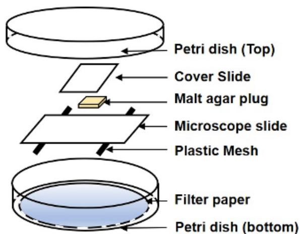
Figure 9. The expanded view of the fungal slide culture.
