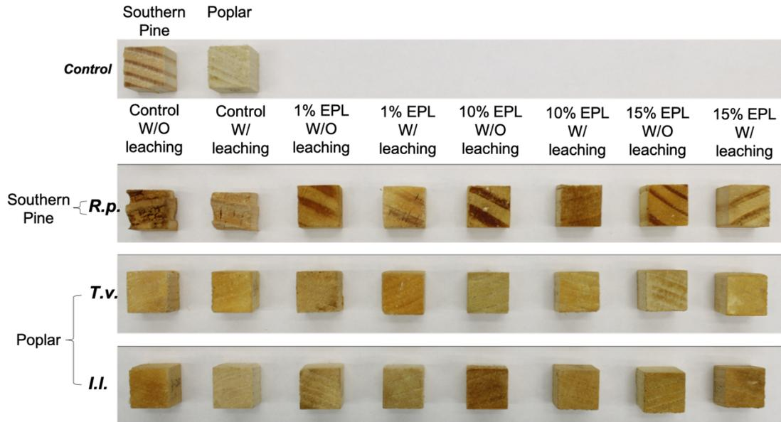
Figure 19. Photographs showing the wood cubes after eight weeks fungal exposure with different treatments.
