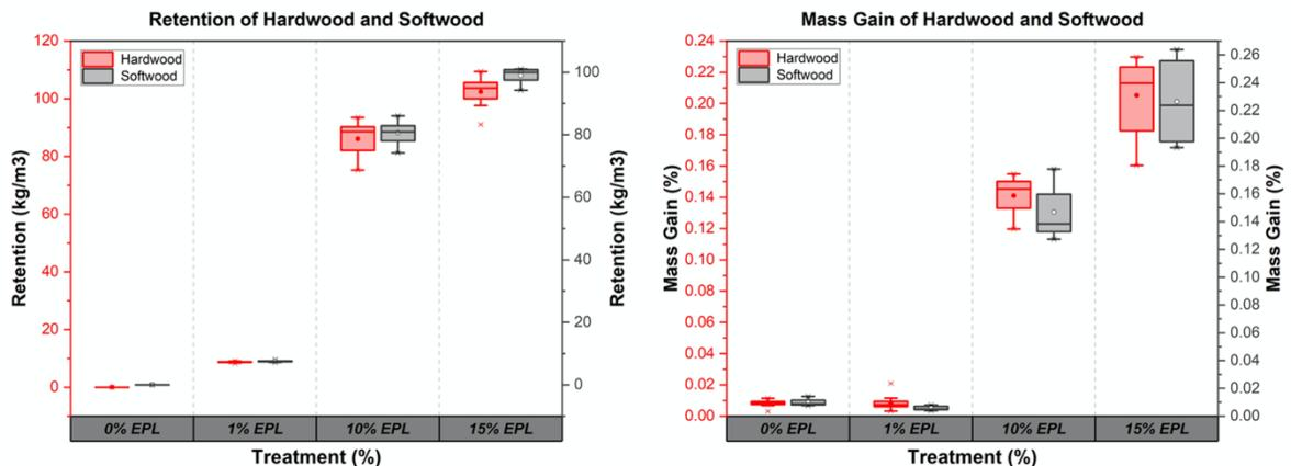
Figure 17. The Retention and mass gain of hardwood and softwood under different treatments.
