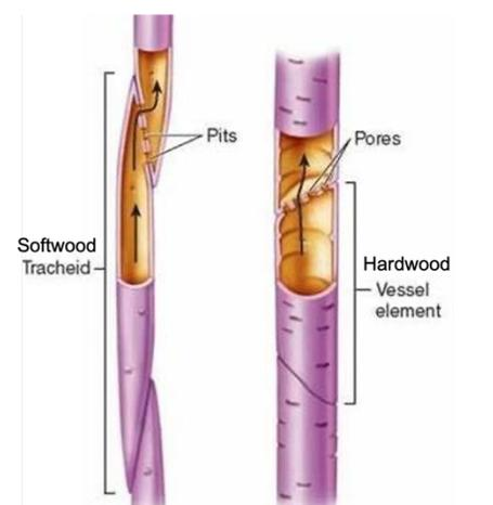
Figure 2. The components of wood cell for tracheid (softwoods) and vessel (hardwoods). The black arrows showed water movement inside the wood cells (Chopite, 2016).
