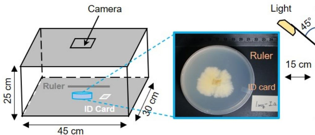
Figure 8. Schematic drawing of the customized box (left), the layout of a Petri dish, ruler and sample ID card inside the box (middle) and light source (right) for photo taking.
