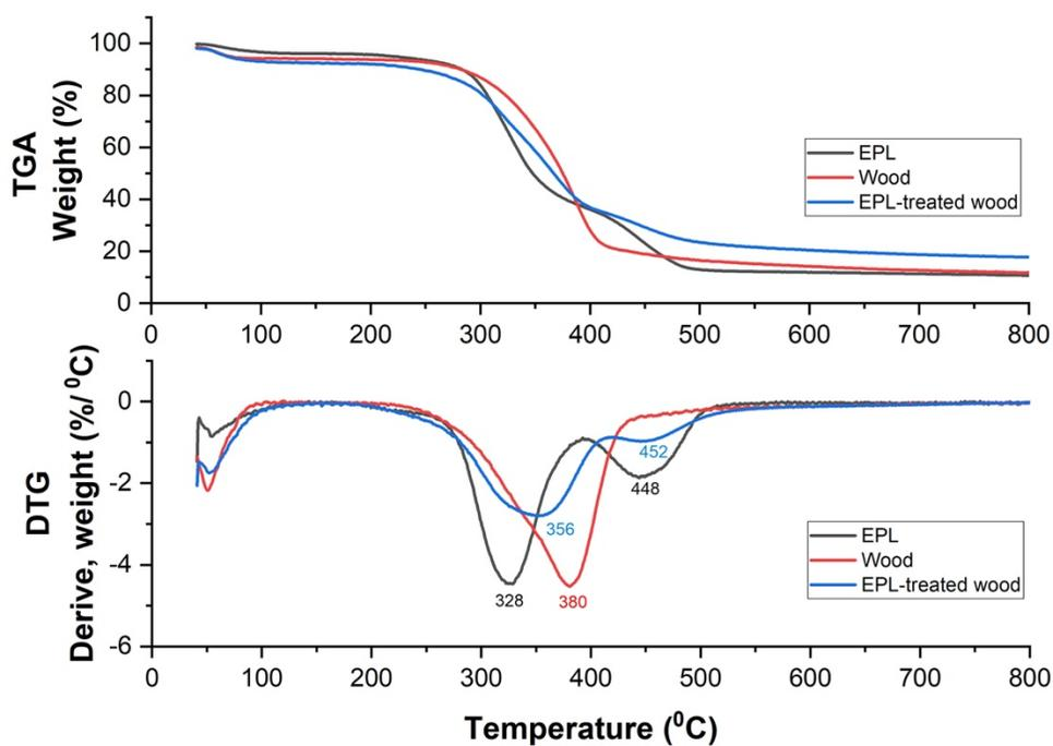
Figure 16. TGA and DTG thermograms of EPL, wood, and EPL-treated wood
