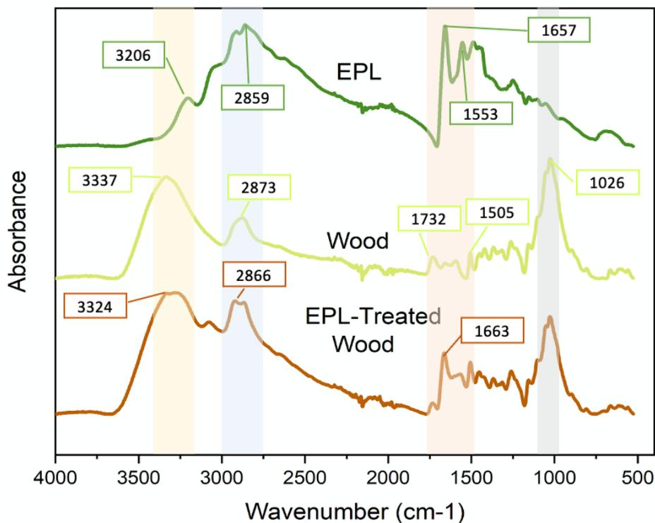
Figure 15. Infrared spectra of EPL, wood, and EPL-treated wood.
