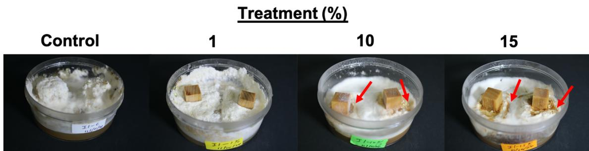
Figure 20. The culture containers showed un-leached poplar wood samples under wood durability test at different EPL treatments percentage. The red arrow indicated the EPL solution leached out at the EPL treatment at 10% and 15%.
