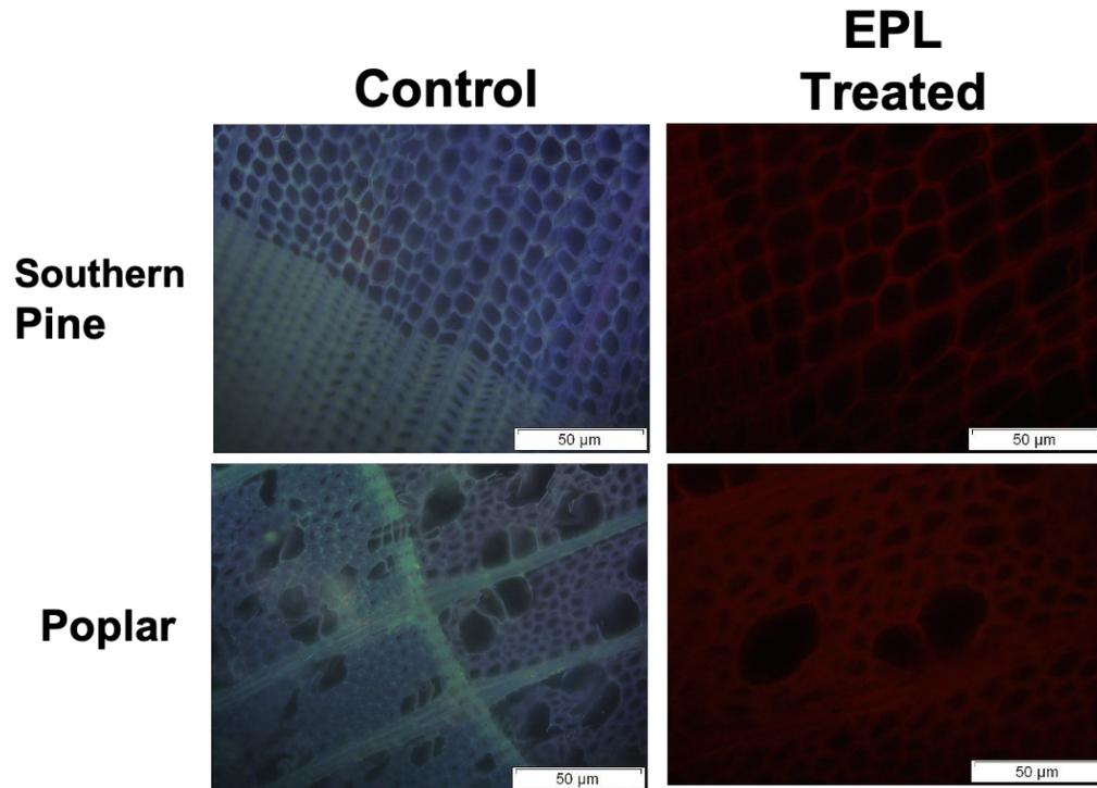
Figure 18. The composition of RGB (filter: BA 515 nm, BA 590 nm, BA 420 nm) light emitted on southern pine and poplar, treated with control and EPL treated under fluorescence microscopy.
