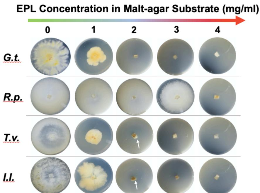
Figure 11. Photographs of four wood-decaying fungi grew on malt-agar substrates amended with 0, 1, 2, 3 and 4 mg/ml of EPL on day 14. The arrows in the Petri dishes represent mycelia colonization.
