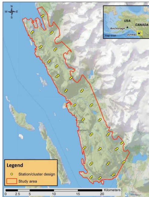
Figure A.1. A map of the study area illustrating the optimized cluster/station layout. The black dots depict two stations per cluster spaced 350 m apart with 3,500 m between each cluster.
