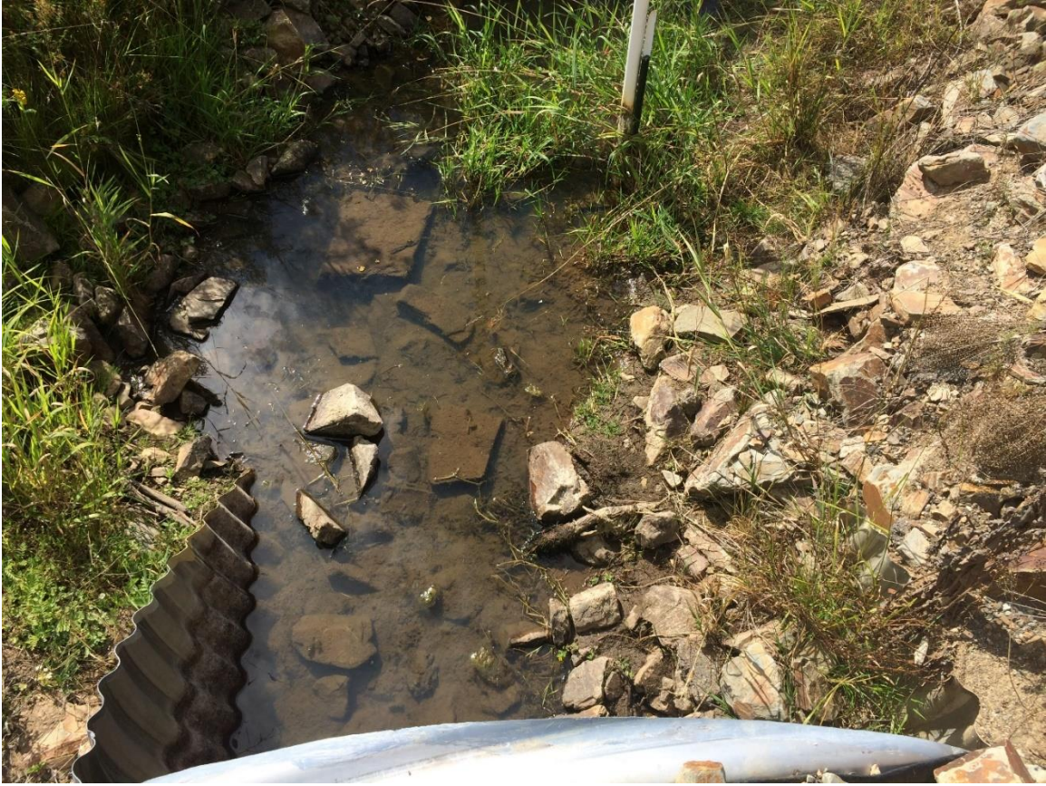
Figure B.3: Picture standing on top of the culvert at the North Side location where cross sections are taken. The pole at the top of the picture is the location of the PVC tube that houses the level logger.
