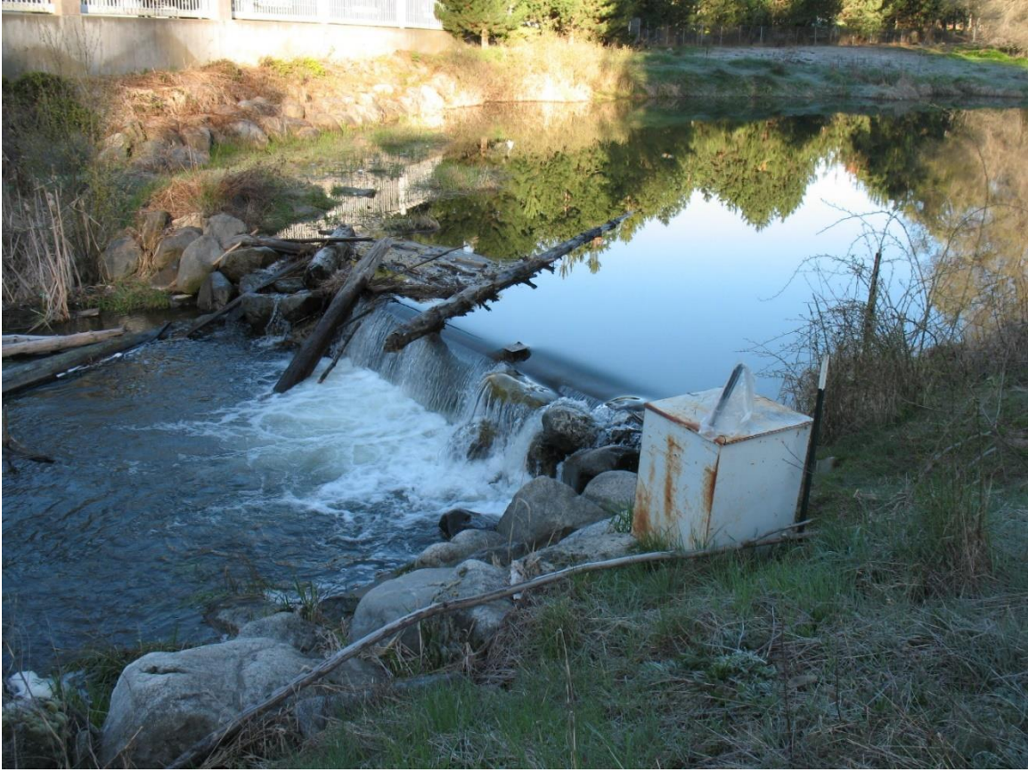
Figure B.5: Picture of the outflow location. The dam is installed and overflowing. The box has a sampler tube that runs across the concrete of the dam. The level logger PVC is barely visible behind the bush on the right side.
