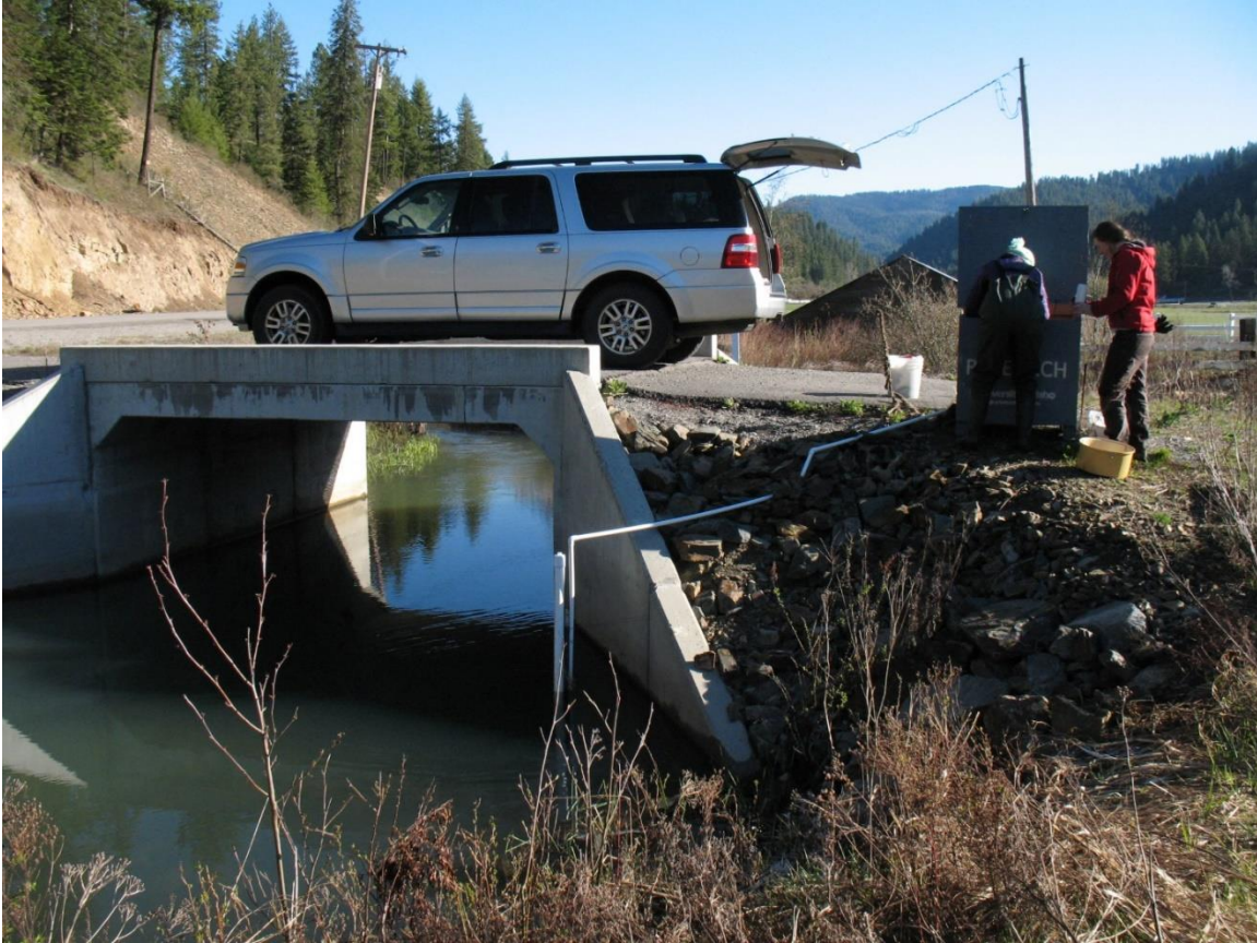
Figure B.4: Picture of the Mike Webb Location. The level logger PVC tube is attached to the intake PVC tube for the sampler. Cross section and velocity measurements were taken at the concrete culvert starting from the right side. Distances were marked on the top of the concrete culvert from 0.2 m to 4.1 m from right to left of the picture.
