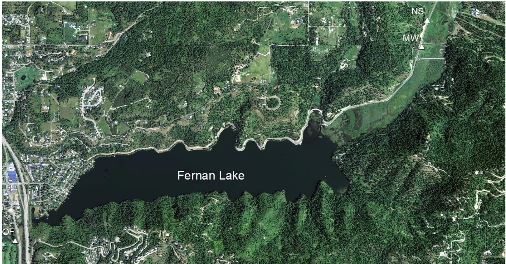
Figure 2.1: Site of automated streamflow samplers (white triangles) on the inflows and outflow of Fernan Lake, Idaho, USA. Image from USGS 2013 0.5m orthoimagery. The North side site (NS) and Mike Webb site (MW) are the two inflow sites and the Outflow site (OF) is the site at the outlet of the lake.
