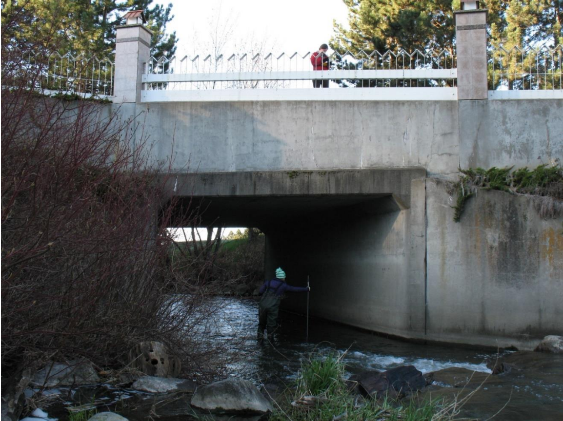
Figure B.8: Image of concrete culvert downstream of the Outflow location (Dam). This is where discharge was measured when the dam was overflowing. Distances were not marked here, a measuring tape was placed on the top of the culvert and the person on the top directed the person below with the velocity meter.
