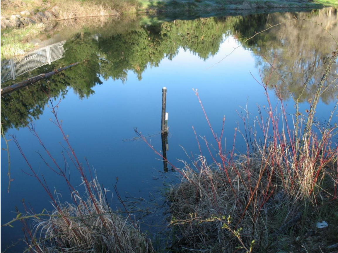
Figure B.9: Image of the Outflow location PVC housing the level logger tube. It is painted black to reduce the effects of ice cover.
