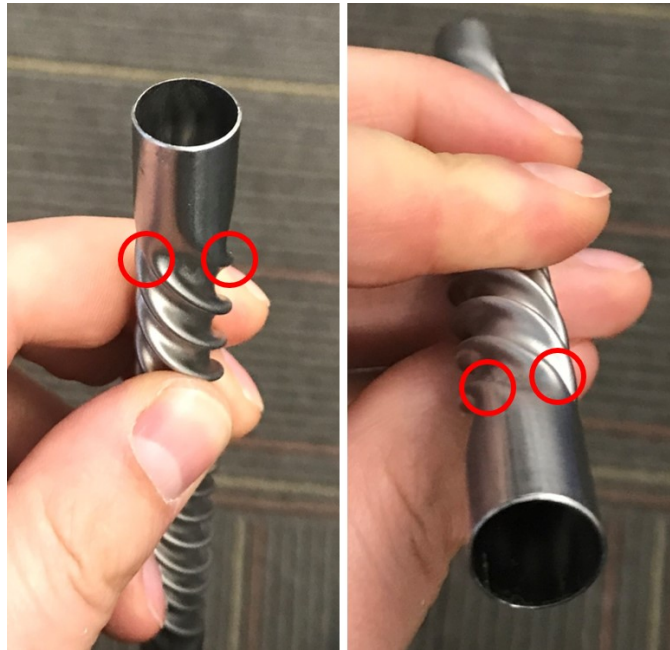
Figure 2.5: The number of starts on the fluted tube.
