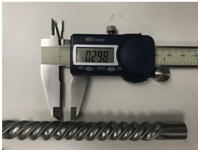
Figure 2.4: The flute pitch on the fluted tube.
