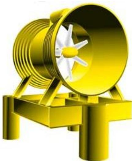
Figure 1-8. Lunar Tidal Turbine by Lunar Energy [16]
