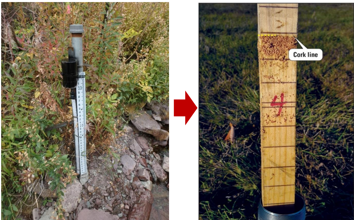
Figure 4: (left) Crest gauge and e-tape installation, (right) high water marked by cork on wooden stake.
