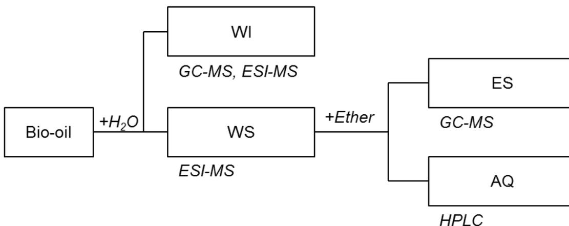
**Figure 6.1** A schematic diagram showing the fractionation and characterization of the bio-oil.
