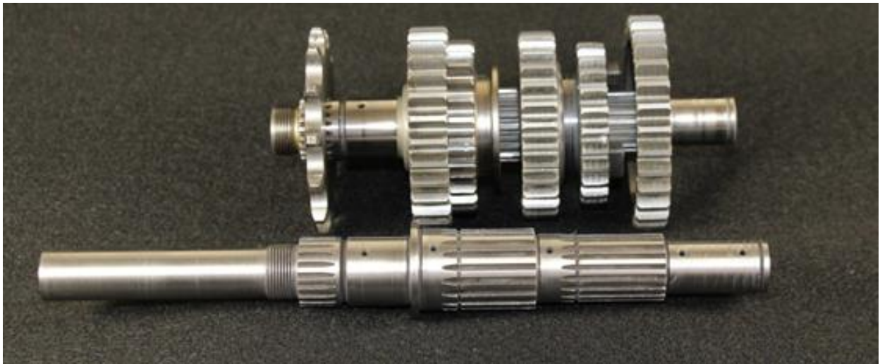
Figure 6: Custom Output Shaft for Post-Transmission Architecture
