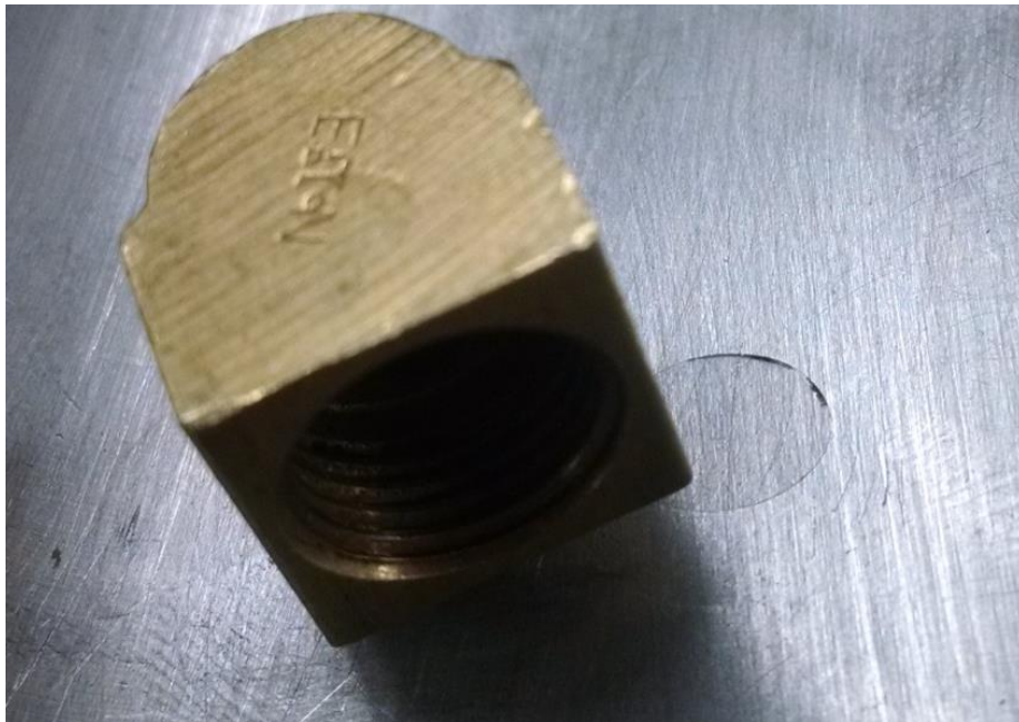
Figure 16: Finished Port for Cross Over Tube
