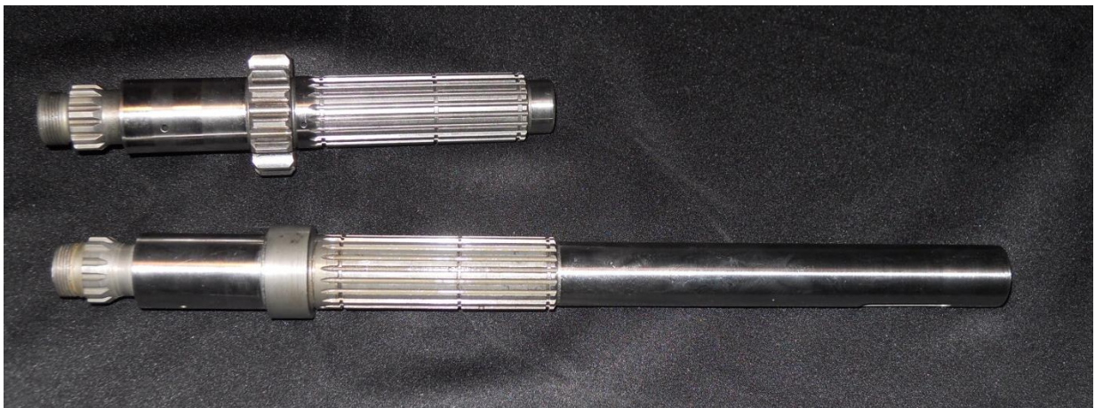
Figure 5: Custom Counter Shaft for Pre-Transmission Architecture
