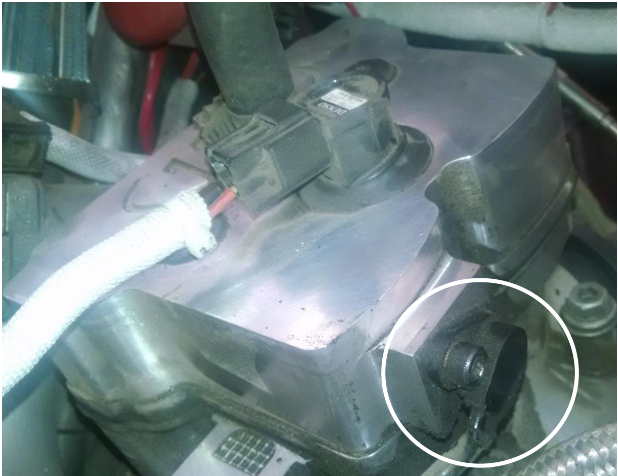
Figure 3: Custom Valve Cover
