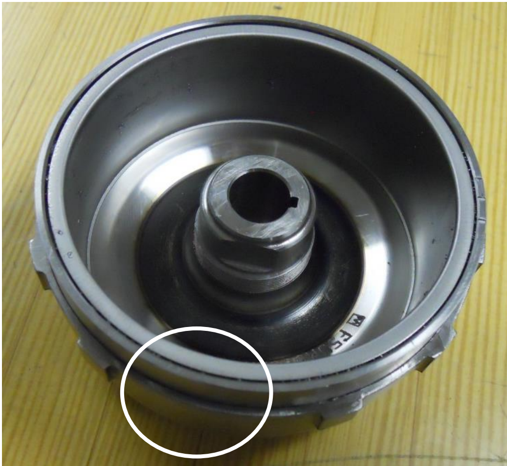
Figure 2: Modified WR250f Flywheel
