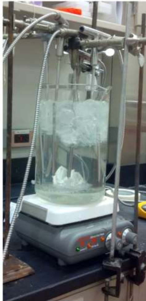
Figure 6. Faulty thermocouple probes in ice bath on top of hot plate to further assess damage.
