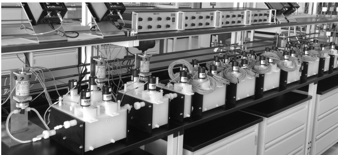
Figure 4.2: INL's 32 stage MEAB mixer-settler system.
